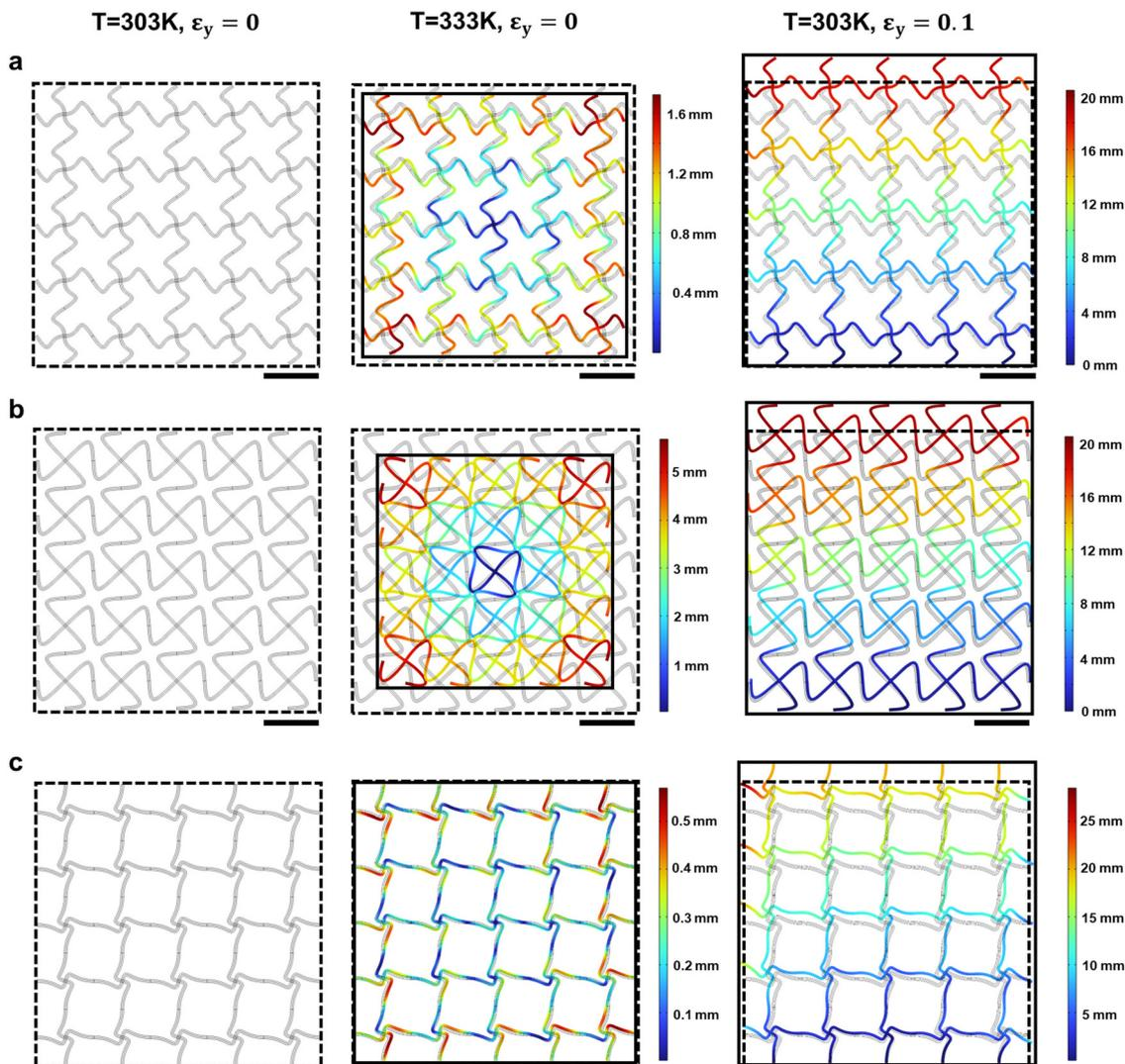
Fig. 3 Numerical simulation results of the BPCM for PR and CTE, scale factor = 4.5: (a) CTE =  $-237.356 \text{ ppm K}^{-1}$ , PR =  $-0.1327$ , (b) CTE =  $-844.864 \text{ ppm K}^{-1}$ , PR =  $-0.0989$  and (c) CTE =  $-31.5737 \text{ ppm K}^{-1}$ , PR =  $-0.5655$  (all the scale bars are 40 mm).
