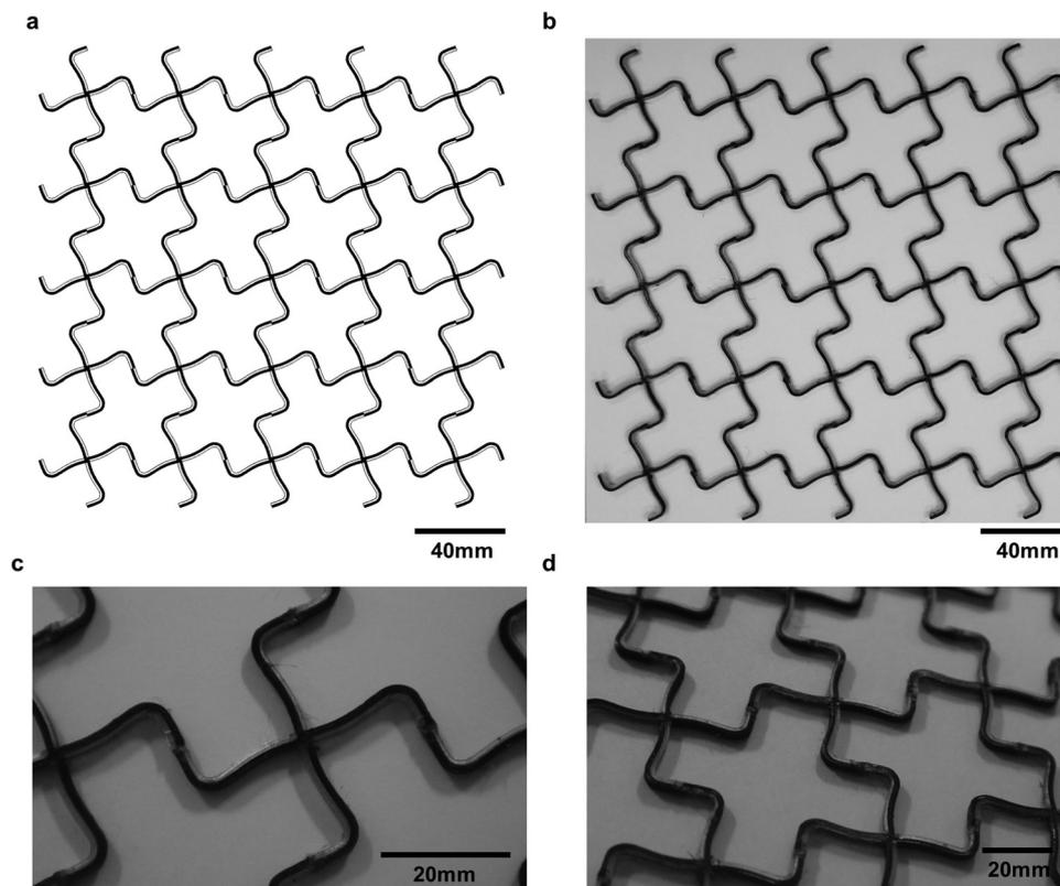
Fig. 2 (a) 2D cross-section image of a representative BPCM and (b)–(d) the fabricated BPCMs via dual nozzle 3D printing.
