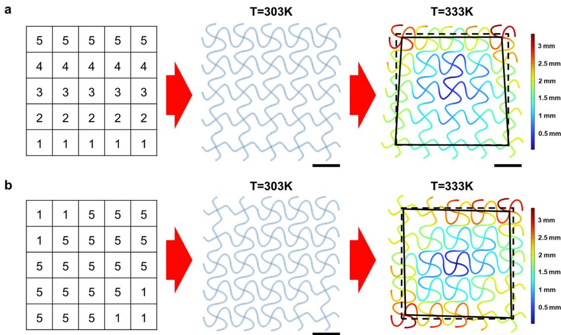
**Fig. 10** Programmable thermal deformation mode with fixed PR, scale factor = 4.5: (a) trapezoidal thermal deformation mode with PR = -0.196 and (b) rhombic thermal deformation mode with PR = -0.18 (all the scale bars are 40 mm).
