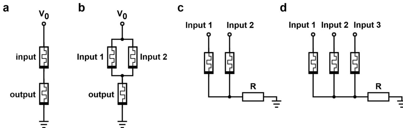
Fig. 3 Schematic of the memristor-based (a) NOT gate, (b) NOR gate, (c) IMP gate, and (d) NAND gate. (a) and (b) Reproduced with permission.<sup>141</sup> Copyright 2017, Springer Nature. (c) and (d) Reproduced with permission.<sup>53</sup> Copyright 2021, Royal Society of Chemistry.
