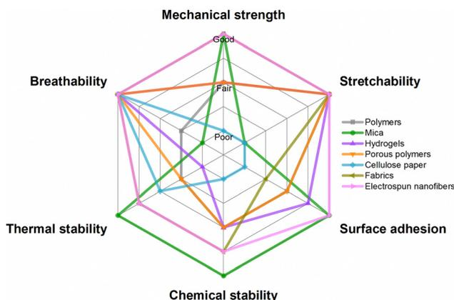
Fig. 2 Properties of different types of flexible substrates.
