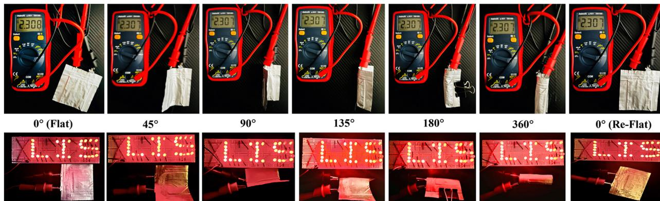
Fig. 6 Upper row: digital pictures of the OCV for the pouch cell consisting of the  $g\text{-C}_3\text{N}_4\text{-Mx/S}$  cathode at different folding angles. Bottom row: pictures of LEDs lighten up by a pouch cell at different folding angles demonstrating the excellent flexible feature of the developed pouch cell.
