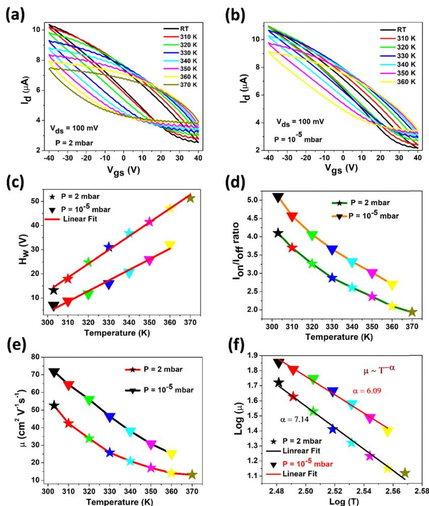
Fig. 4 (a) and (b) Transfer characteristics, (c) hysteresis width, (d) on/off current ratio, (e) and (f) mobility at different temperatures of the BP device under 2 mbar and  $10^{-5}$  mbar pressures. Lines in (d) and (e) are guide to the eye.
