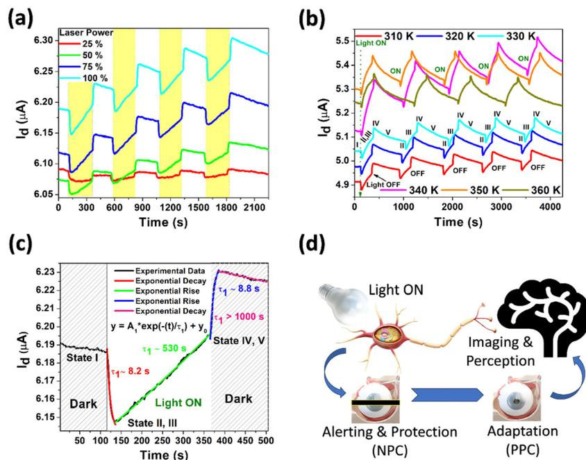
Fig. 6 (a) Transient photocurrent at different laser powers at 310 K,  $V_{ds} = 10$  mV. (b) Transient photocurrent at different temperatures with a maximum laser power, at  $V_{ds} = 100$  mV. In both cases, the maximum laser power was 110 mW,  $10^{-5}$  mbar pressure, and  $V_{gs} = 0$  V. (c) Current decay/rise and exponential fit at 310 K,  $10^{-5}$  mbar pressure. (d) Corresponding illustration of the obtained NPC and PPC for neuromorphic vision sensors.
