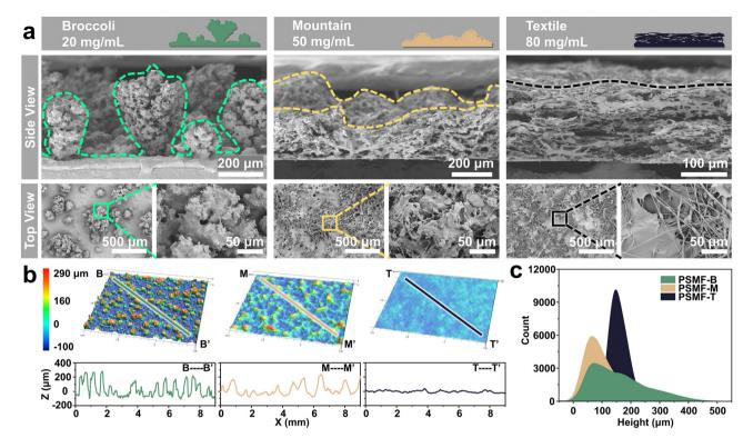
Fig. 2 Morphological characteristics of PSMFs. (a) SEM images of PSMFs on the view of side, and top. (b) 3D surface profile measurement results of the PSMFs (7.56 mm  $\times$  5.67 mm) and height of the specific lines. (c) Height distribution of PSMFs (7.56 mm  $\times$  5.67 mm).
