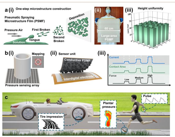
Fig. 1 Overview of the large-area sensor array based on PSMF. (a-i) Schematic of the PSMF mechanism; (a-ii) a PSMF of about  $60 \times 60 \text{ cm}^2$  large-area; (a-iii) height uniformity of the constructed PSMF. (b-i) Sensor array for pressure distribution detection; (b-ii) schematic diagram of a single sensing unit structure; (b-iii) correspondence of sensor output and input. (c) Diversified applications under different pressure ranges that the fabricated sensor is qualified.
