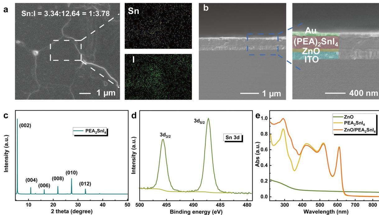
Fig. 2 (a) Top-view SEM image of  $\text{PEA}_2\text{SnI}_4$  and mapping images for the corresponding elements (Sn and I). (b) Cross-sectional image of the  $\text{PEA}_2\text{SnI}_4/\text{ZnO}$  device. (c) XRD pattern of  $\text{PEA}_2\text{SnI}_4$  film. (d) XPS spectra of  $\text{PEA}_2\text{SnI}_4$ : Sn 3d. (e) Absorption spectrum of ZnO,  $\text{PEA}_2\text{SnI}_4$ , and the  $\text{PEA}_2\text{SnI}_4/\text{ZnO}$  films.
