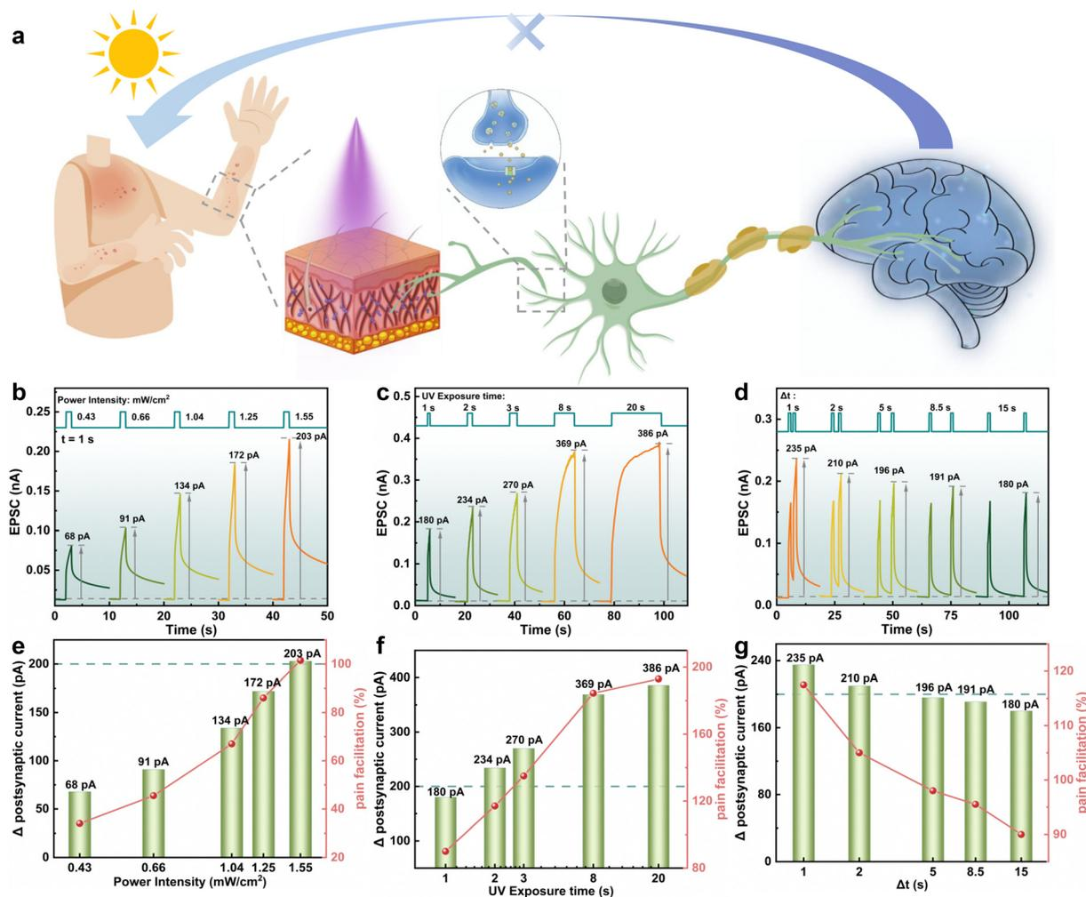
**Fig. 4** (a) Schematic diagram of the device detecting, recognizing, and self-protecting against UV stimuli. (b) EPSC and (e)  $\Delta$ PSC and pain facilitation under different UV irradiation intensities (320 nm, pulse width of 1 s). (c) EPSC and (f)  $\Delta$ PSC and pain facilitation under different UV irradiation times (320 nm, 1.25 mW cm<sup>-2</sup>). (d) EPSC and (g)  $\Delta$ PSC and pain facilitation under different UV irradiation intervals (320 nm, 1.25 mW cm<sup>-2</sup>).
