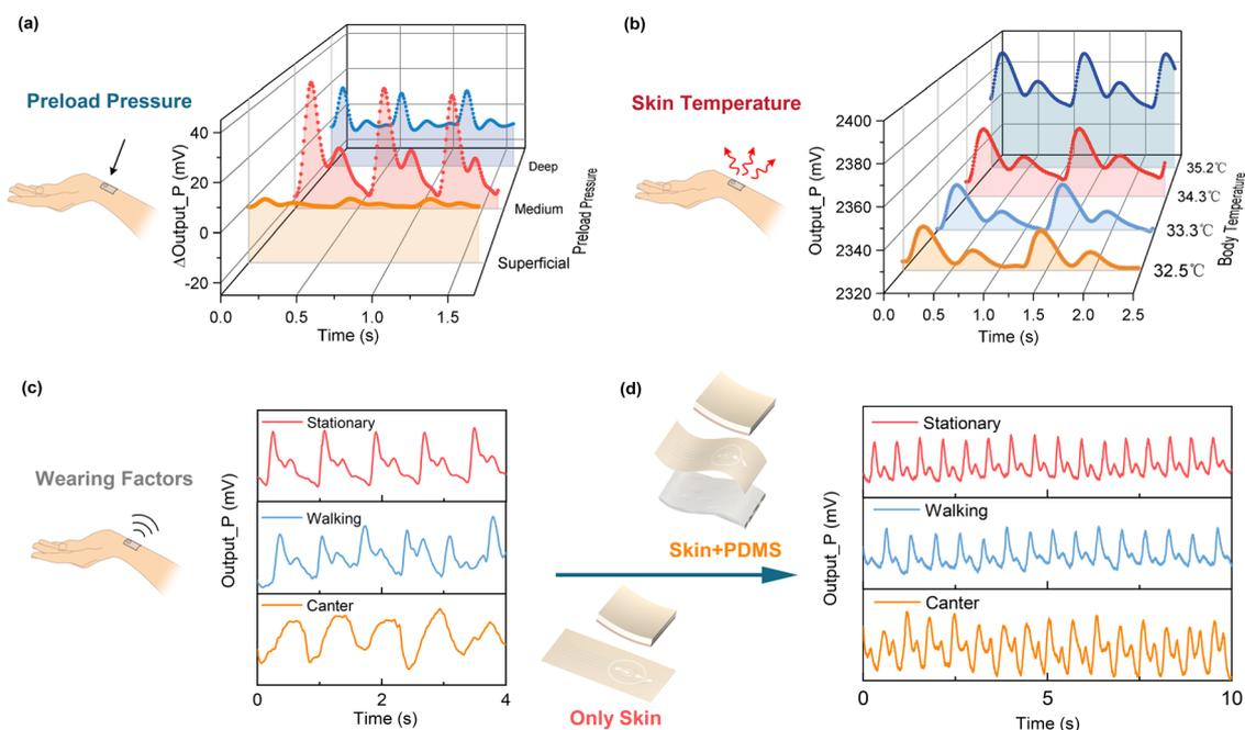
Fig. 3 Factors influencing the pulse wave measurement. (a) Effects of preload pressures on the pulse wave measurement. (b) Effects of skin temperatures on the pulse wave measurement. (c) Effects of body movements on the pulse wave measurement using the pulse sensor with only human skin. (d) Effects of body movements on the pulse wave measurement using the pulse sensor with a combination of human skin and porous PDMS/Ag.
