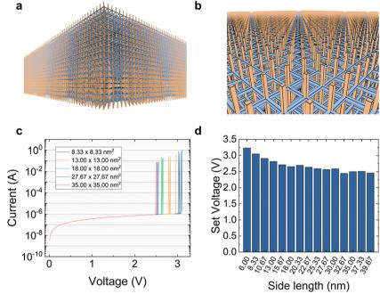
Fig. 5 (a) Resistance network corresponding to a great area (100 nm  $\times$  100 nm) device. (b) Resistance network corresponding to a great area (100 nm  $\times$ 100 nm) device (zoomed-in view) (c) Several simulated set I-V curves for different device areas (the current values are scaled with respect to the lowest area shown in the plot, i.e. (8.33 nm  $\times$  8.33 nm)). (d) Set voltage versus device side length (assuming a device square area obtained as (side length)<sup>2</sup>).
