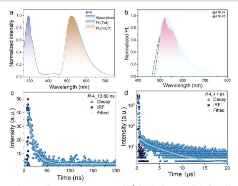
Fig. 4 (a) UV-vis spectra and PL spectra of  $\it R-4$  measured in toluene solution ( $\it 10^{-5}$  M) and 5 wt% doped in mCP film ( $\it \lambda_{ex}$  = 420 nm); (b) low-temperature fluorescence (Fl) and phosphorescence (Ph) of  $\it R-4$  doped in mCP film ( $\it \lambda_{ex}$  = 370 nm, delayed 2 ms); and (c) and (d) transient PL decay curves ( $\it \lambda_{ex}$  = 420 nm) of 5 wt%  $\it R-4$  doped in mCP film.
