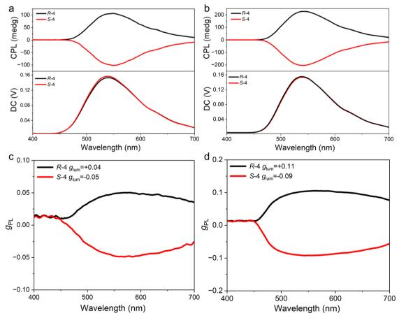
Fig. 5 (a) CPL spectra and (c)  $g_{lum}$  values of CPL versus wavelength of **R/S-4** in neat films; (b) CPL spectra and (d)  $g_{lum}$  values of CPL versus wavelength of **R/S-4** in doped mCP films ( $\lambda_{ex} = 340$  nm).
