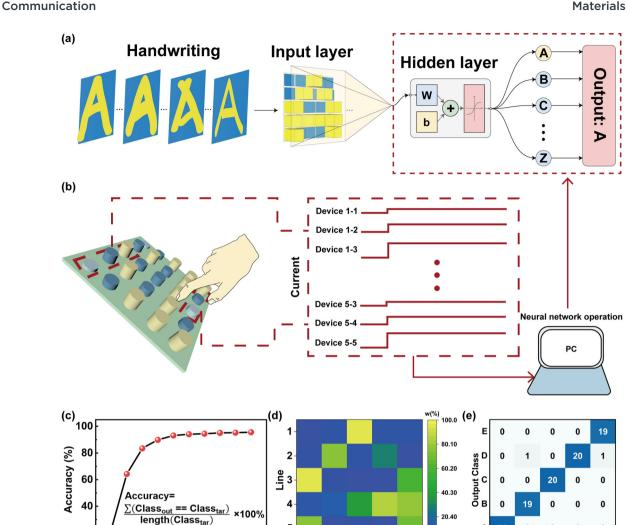
Fig. 6 (a) A schematic of handwriting recognition based on in-sensor computing. (b) The structure and working principle of the humidity in-sensor handwriting recognition system. (c) The accuracy of handwriting recognition. (d) The weight of  $5 \times 5$  array after handwriting. (e) The confusion graph of the output class and the target class about handwriting letters of alphabet "A," "B," "C," "D," and "E" after 40 cycles.
