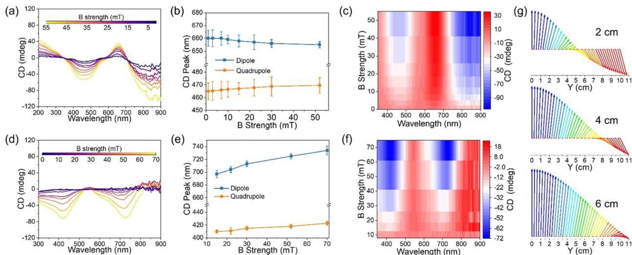
**Fig. 3** (a)–(f): CD spectra (a) and (d), the corresponding dipole and quadrupole peak shifts (b) and (e), and the peak intensity changes (c) and (f) of Ag@Fe<sub>3</sub>O<sub>4</sub> nanoparticle assembly under  $B_x$  and  $B_y$  with varying strengths. (g) Simulated magnetic field vector rotation along the Y-axis under different distances (2, 4, 6 cm) along the X-axis from the magnet, showing that chirality decreases with increasing separation distance.
