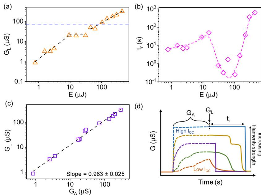
Fig. 4 Analysis of the  $G$  profile. (a) Variation of  $G_L$  and (b)  $t_r$  as a function of the electrical energy stress ( $E$ ) on the device. (c) Variation of  $G_L$  with  $G_A$ . (d) Schematic of a typical  $G$  profile ( $G$  evolution during pulsing and retention after pulsing) visualised at different ranges of  $I_{CC}$  under similar pulsing conditions ( $V_p \sim 1$  V,  $V_R \sim 10$  mV,  $t_i$  and  $t_w \sim 50$  ms).
