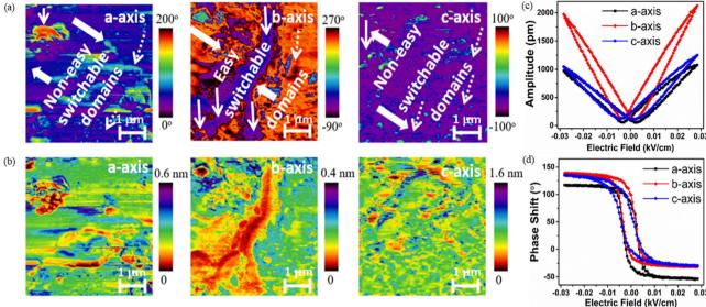
Fig. 2 (a) Vertical PFM phase images recorded on a single crystal of  $\bf 1$  oriented along a-, b- and c-axis and (b) corresponding amplitude images showing the different domains, (c) amplitude vs. electric field butterfly loop, (d) phase shift vs. electric field hysteresis loop along the three directions (applied voltage is normalized with respect to electric field).
