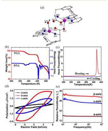
Fig. 1 (a) Ball and stick representation of crystal structure of 1. The Hydrogen atoms are omitted for clarity, (b) TGA-DTA thermograms of 1, (c) DSC curves of 1, (d) and (e) direction dependent polarization vs. electric field (P-E) hysteresis loop and relative permittivity  $(\varepsilon_{\rm r}')$  vs. frequency  $(10^3-10^6 \text{ Hz})$  measured along a, b and c-axes respectively on a single crystal of **1**.
