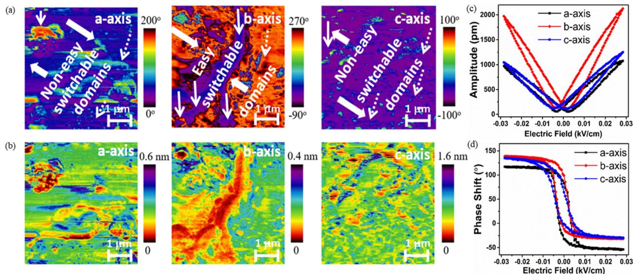
Fig. 2 (a) Vertical PFM phase images recorded on a single crystal of **1** oriented along *a*-, *b*- and *c*-axis and (b) corresponding amplitude images showing the different domains, (c) amplitude vs. electric field butterfly loop, (d) phase shift vs. electric field hysteresis loop along the three directions (applied voltage is normalized with respect to electric field).
