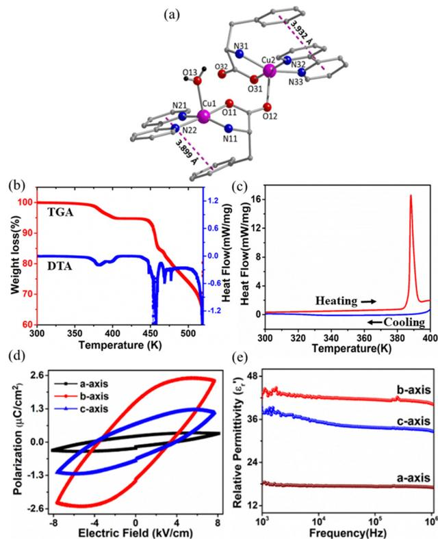
**Fig. 1** (a) Ball and stick representation of crystal structure of **1**. The Hydrogen atoms are omitted for clarity, (b) TGA–DTA thermograms of **1**, (c) DSC curves of **1**, (d) and (e) direction dependent polarization vs. electric field ( $P$ – $E$ ) hysteresis loop and relative permittivity ( $\epsilon_r'$ ) vs. frequency ( $10^3$ – $10^6$  Hz) measured along *a*, *b* and *c*-axes respectively on a single crystal of **1**.
