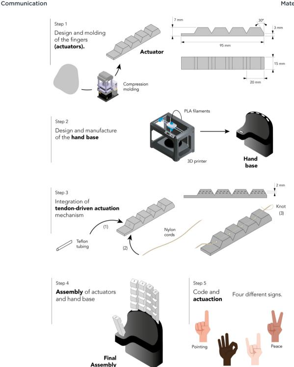
Fig. 2 Schematic representation of soft robotic gripper assembly.
