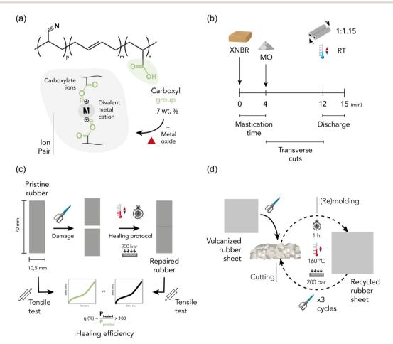
(a) Structure of XNBR and ion pairs, (b) mixing, (c) self-healing, and (d) recycling protocol.
