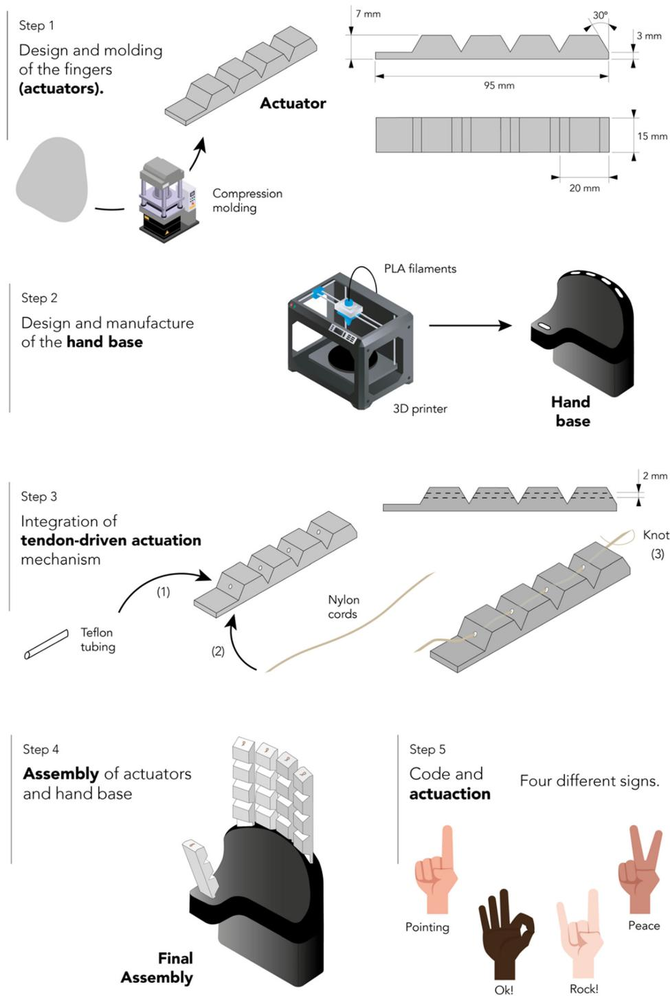
Fig. 2 Schematic representation of soft robotic gripper assembly.
