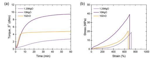
Fig. 4 (a) Curing curves (160 °C) and (b) mechanical properties of the cured ionic elastomers.
