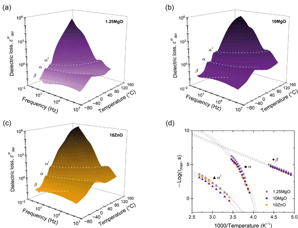
Fig. 5 3D plots of conduction-free dielectric loss ( $\epsilon''_{\text{der}}$ ) with respect to temperature and frequency for (a) 1.25MgO, (b) 10MgO and (c) 10ZnO. (d) Activation plot of the ionic elastomers.
