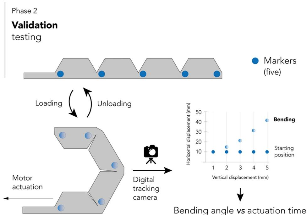
Fig. 3 Schematic representation of the validation testing.
