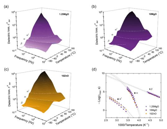
Fig. 5 3D plots of conduction-free dielectric loss ( $\epsilon_{der}''$ ) with respect to temperature and frequency for (a) 1.25MgO, (b) 10MgO and (c) 10ZnO. (d) Activation plot of the ionic elastomers.
