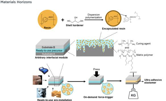
Fig. 1 Illustration of the on-demand ultra-high adhesion formation of the ready-to-use precursor and its preparation process. The resin, curing agent, and matrix polymer are MDI-prepolymer, PPG-diamine, and acrylates copolymer, respectively.
