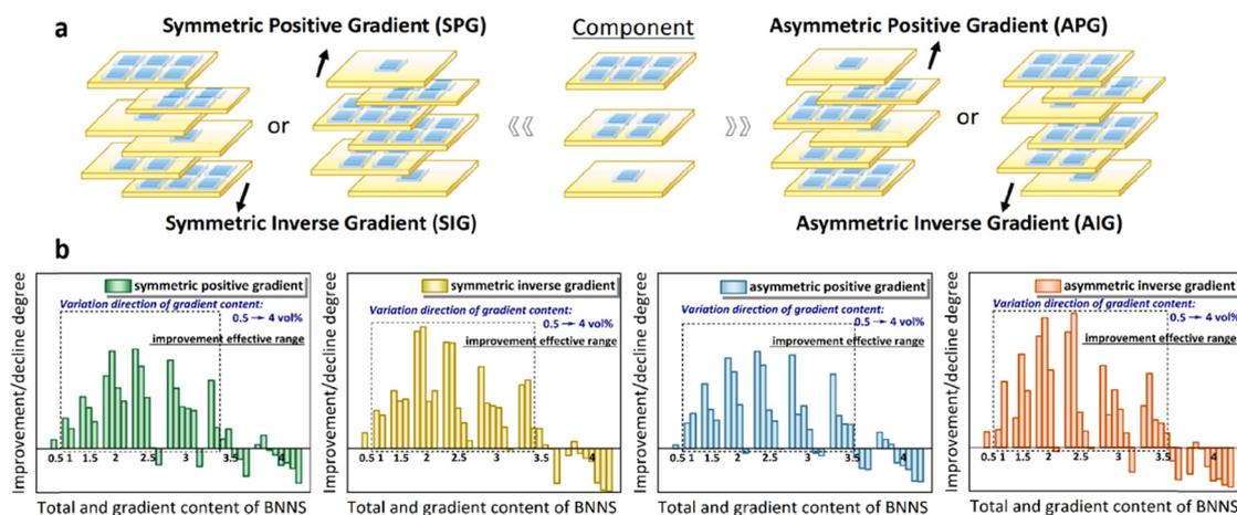
Fig. 1 (a) Design concept of PEI-based composite dielectrics with different topological gradient structures. (b) Improvement or decline degree of all composite structures compared with the matrix.
