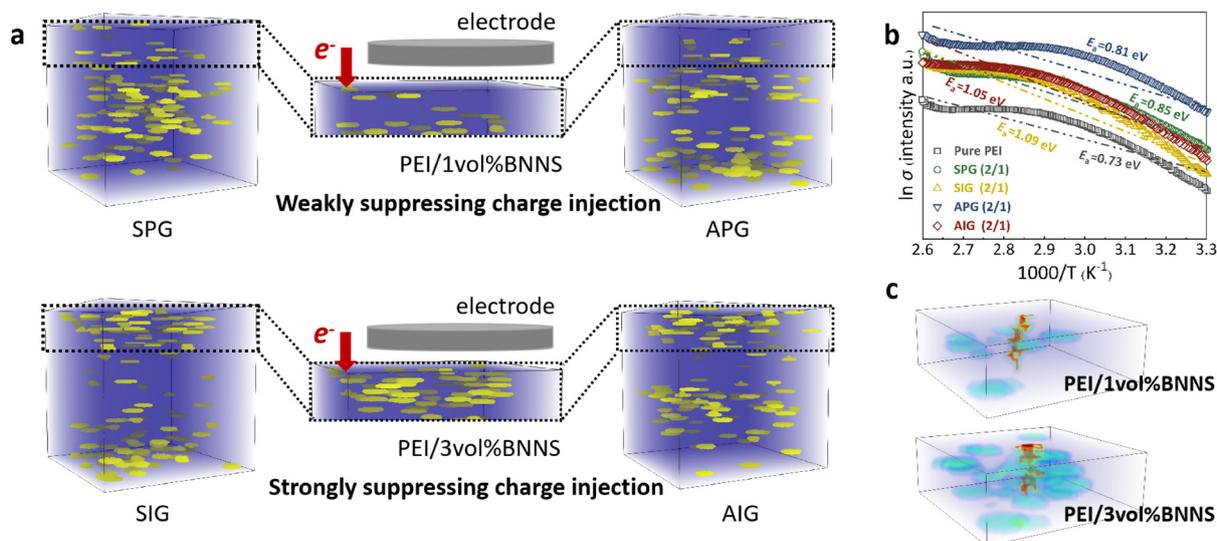
Fig. 5 (a) Schematic diagram of the metal/dielectric interface. (b) Dependence of  $\ln \sigma$  on  $1000/T$  for the pure PEI, SPG (2/1), SIG (2/1), APG (2/1), and AIG (2/1) composite dielectrics at  $10^2$  Hz. (c) Development of the breakdown path in the surface barrier layer.
