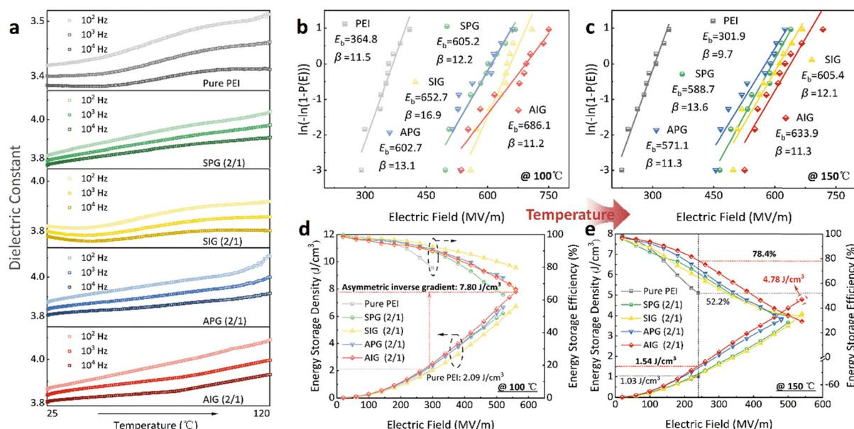
Fig. 7 (a) The temperature dependence of the dielectric constant of pure PEI, and SPG (2/1), SIG (2/1), APG (2/1), and AIG (2/1) composite dielectrics at  $10^2$ ,  $10^3$ , and  $10^4$  Hz. The breakdown strength of pure PEI, and SPG (2/1), SIG (2/1), APG (2/1), and AIG (2/1) composite dielectrics at (b) 100 °C and (c) 150 °C. The energy storage density and efficiency of pure PEI, and SPG (2/1), SIG (2/1), APG (2/1), and AIG (2/1) composite dielectrics at (d) 100 °C and (e) 150 °C.
