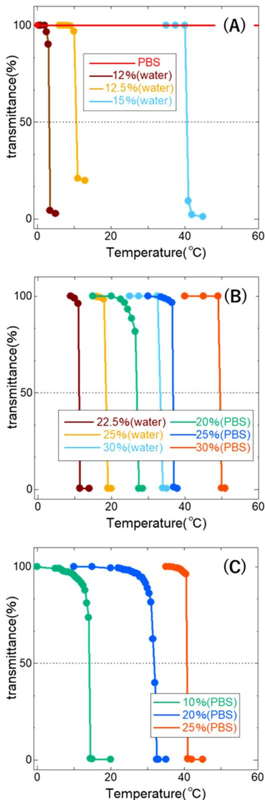
**Fig. 1** Changes in transmittance intensity across different temperature ranges (UV-vis,  $\lambda = 550$  nm; 50% transmittance indicates phase separation temperature). (A) The phase separation temperatures for different polymer concentrations of PLL-SA50 in pure water. (B) The phase separation temperatures for different polymer concentrations of PLL-PA50 in pure water and PBS. (C) The phase separation temperatures for PLL-PA(-SH) at various concentrations in PBS.
