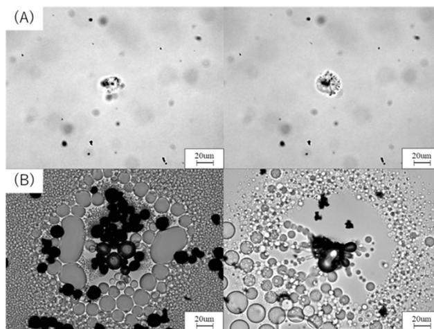
**Fig. 4** Laser microscopy images ( $\lambda = 808$  nm, irradiation: 3 s, scale: 20  $\mu$ m): (A) MHDA + LMNPs solution, and (B) composite.
