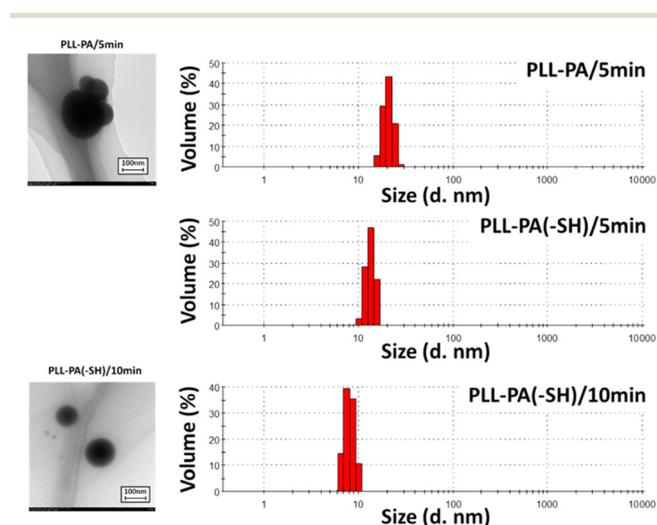
**Fig. 2** TEM images and DLS measurements demonstrating LM nanoparticle formation and thiolation via pulse sonication with 2 s of irradiation per pulse (20 kHz, ice bath, 10 mL polymer solution, 30  $\mu$ L LM).
