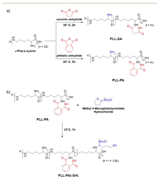
Scheme 1 Synthesis of (a) PLL-PA and (b) PLL-PA(-SH).
