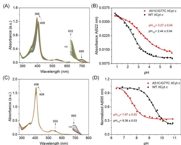
**Fig. 5** Alkaline conformational transition and acidic unfolding studies on WT and A51C/G77C *hCyt c*. (A) pH-dependent UV-vis spectra changes of A51C/G77C *hCyt c* in acidic unfolding studies; (B) plots of 622 nm versus pH for acid unfolding of WT and A51C/G77C *hCyt c*; (C) pH-dependent UV-vis spectra changes of A51C/G77C *hCyt c* in alkaline transition studies; (D) normalized absorbance at 695 nm in the alkaline pH range.
