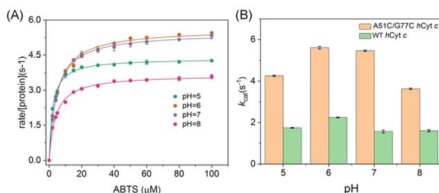
Fig. 9 Peroxidase activity assay using ABTS as a substrate. (A) Michaelis–Menten plots vs. the concentrations of ABTS for A51C/G77C *hCyt c* at pH 5–8. (B)  $k_{\text{cat}}$  vs. pH values for A51C/G77C and WT *hCyt c*. The error bars are based on the standard deviation of six independent experiments. The reaction was initiated by mixing 200 mM  $\text{H}_2\text{O}_2$  with 10  $\mu\text{M}$  protein in 50 mM potassium phosphate buffer at room temperature.
