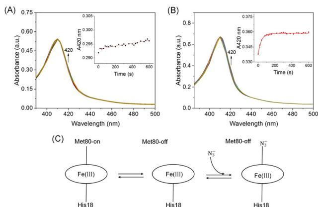
**Fig. 6** UV-vis spectra of (A) WT and (B) A51C/G77C *hCyt c* (10 μM) upon mixing with NaN<sub>3</sub> (200 mM) in 100 mM potassium phosphate buffer (pH 7.0) at room temperature. The absorption at 420 nm was recorded to calculate the *k*<sub>obs</sub>. Time-dependent change of the Soret band is shown as an inset. (C) Proposed mechanism for azide binding to the heme iron of *Cyt c*.
