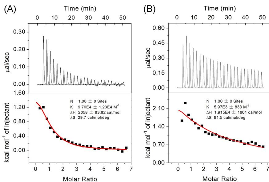
**Fig. 10** Representative ITC thermograms of (A) WT and (B) A51C/G77C *hCyt c* titrated into the solution of *hNgb*. Both samples were prepared in a 10 mM potassium phosphate solution (pH 7.0). The data were fitted to the OneSites binding model.
