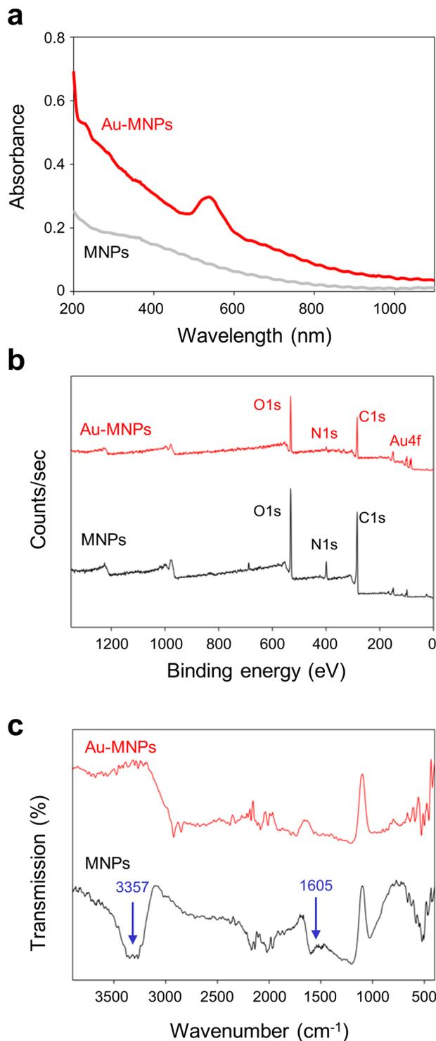
Fig. 2 Characterization of gold-melanin nanoparticles. Absorption (a), X-ray photoelectron (XP) (b), and Fourier transform-infrared (FT-IR) (c) spectra of MNPs and Au-MNPs.
