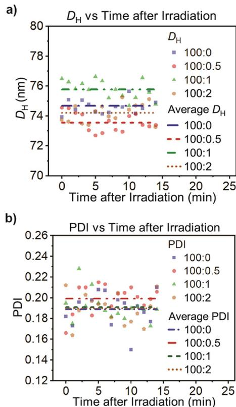
**Fig. 7** a) Hydrodynamic diameter ( $D_H$ ) and b) polydispersity index (PDI) of the polymersomes with different amounts of motors after 5 min of light irradiation at 24 °C. Cumulant fit error bars are smaller than the symbol size and were omitted for clarity.
