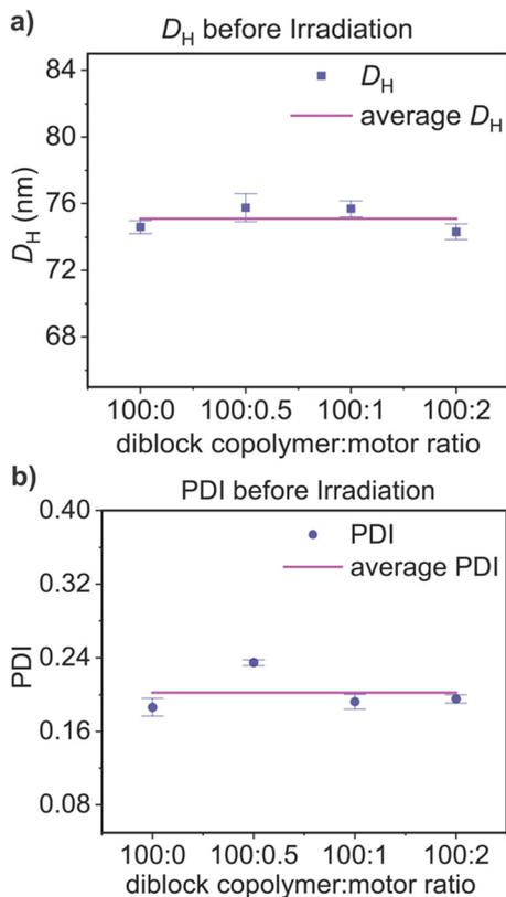
**Fig. 6** a) Hydrodynamic parameter ( $D_H$ ) and b) polydispersity index (PDI) of polymersomes with different concentrations of motors without light irradiation. DLS measurements were collected at 22 °C.
