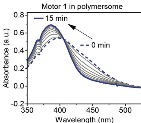
Fig. 9 UV-vis absorption spectra showing the thermal helix inversion of motor 1 incorporated in polymersomes. Metastable **1b** (dash line) was formed after irradiation with 370 nm for 5 min. Over time, **1b** converts into **1c** (solid line).
