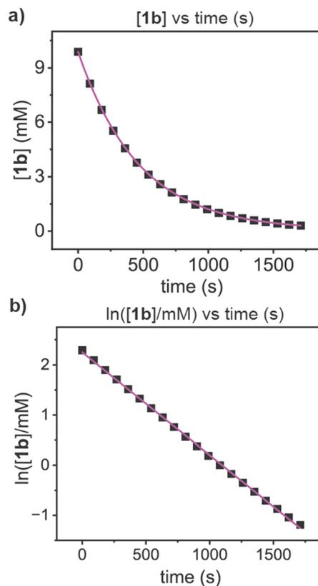
**Fig. 3** (a) Decrease in the concentration of metastable 1b over time measured by  $^1\text{H}$  NMR spectroscopy in chloroform-d. (b) First-order kinetic analysis of the NMR data. The slope of the linear fit gives the THI rate constant ( $k$ ) of 0.00205  $\text{s}^{-1}$  at 20 °C.
