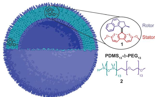
Fig. 1 Molecular motor, **1**, in the hydrophobic region of the bilayer of a polymersome formed by the self-assembly of PDMS<sub>13</sub>-*b*-PEG<sub>13</sub> diblock copolymer **2**. Created with BioRender.
