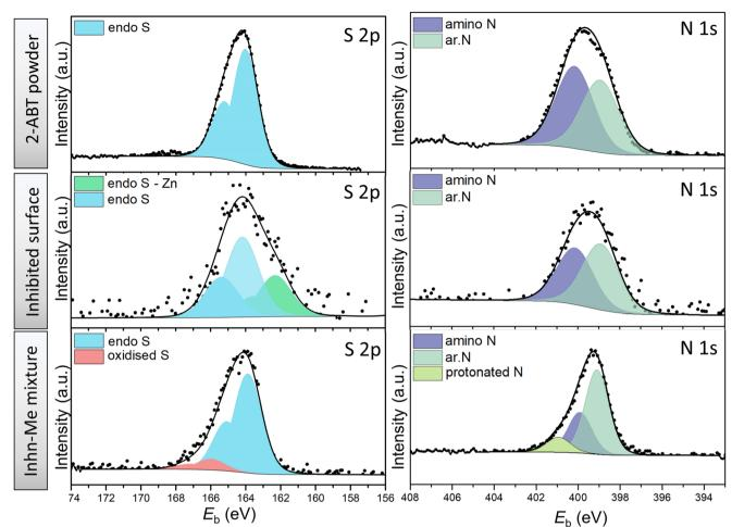
Fig. 5 High-resolution XPS spectra of S 2p and N 1s of 2-ABT powder (reference), ZE surface treated with 2-ABT and precipitates of inhibitor solution mixed with ZnCl<sub>2</sub>
