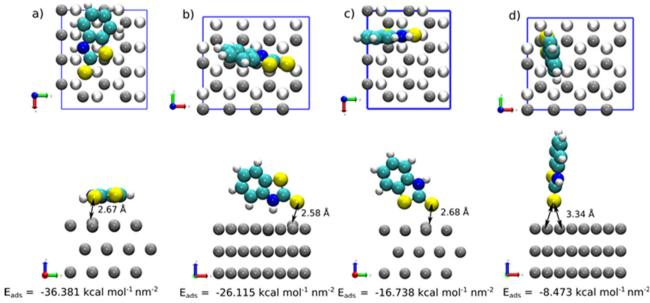
Fig. 8 Top view and side view of the final adsorption structures at low concentration (1 molecule per nm<sup>2</sup> obtained for 2-MBT on Zn{0001}: (a) parallel, (b) (S,NH)-Zn, (c) (S,S)-Zn, and (d) (S)-Zn cases. White, cyan, yellow, blue, and gray colored spheres represent H, C, S, N, and Zn atoms, respectively. In the top view, degraded color spheres represent the Zn under the surface.
