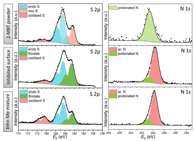
Fig. 6 High-resolution XPS spectra of S 2p and N 1s of 2-MBT powder (reference), ZE surface treated with 2-MBT and precipitates of inhibitor solution mixed with ZnCl<sub>2</sub>.
