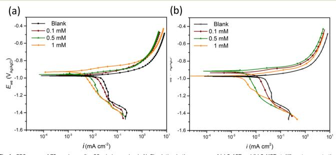
Fig. 1 PDS curves of ZE specimen after 90 min immersion in NaCl solution in the presence of (a) 2-ABT and (b) 2-MBT at different concentrations (0-1 mM).
