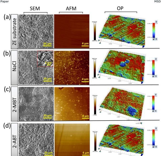
Fig. 4 Surface morphology at different resolutions of ZE specimens under different corrosive conditions. (a) ZE substrate, (b) ZE after 90 min immersion in 0.1 M NaCl, (c) and (d) ZE specimens after 90 min immersion in 0.1 M NaCl in the presence of 1 mM 2-MBT and 2-ABT, respectively.
