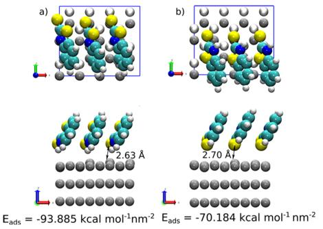
Fig. 9 Top view and side view for the final adsorption structures at high concentration (3 molecules per nm<sup>2</sup> obtained for 2-MBT on Zn{0001}: a) (S,NH)-Zn, and b) (S,S)-Zn cases. White, cyan, yellow, blue, and gray colored spheres represent H, C, S, N, and Zn atoms, respectively. On the top view of each case, degraded color spheres represent the Zn under the surface.
