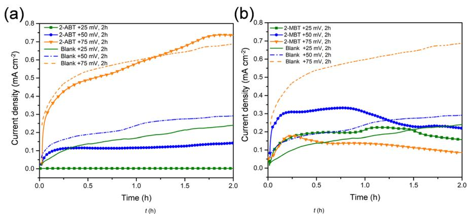
**Fig. 10** Variation of current densities of ZE interface as a function of time under different applied overpotentials in the inhibitor (1 mM)-containing NaCl solution. (a) 2-ABT and (b) 2-MBT.
