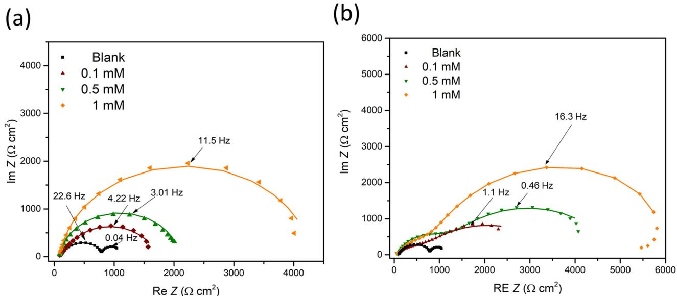
Fig. 2 EIS diagrams of ZE specimen after 90 min immersion in NaCl solution with inhibitor at different concentrations (0–1 mM). (a) 2-ABT; (b) 2-MBT.
