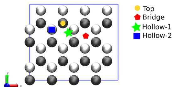
Fig. 7 Different adsorption sites at the Zn-{0001} plane. Top (yellow circle), bridge (red pentagon), hollow-1 (green star), and hollow-2 (blue square) represent the different possible adsorption sites. Gray-colored spheres: Zn surface; degraded color spheres: Zn under surface.
