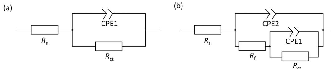
Fig. 3 EEC models used for EIS fitting.  $R_s$ ,  $R_f$  and  $R_{ct}$  are the resistance of the solution, inhibitor/product film, and charge transfer, respectively. (a) CPE1 is the constant phase element simulating the double layer capacitance, and (b) CPE2 represents the response of inhibitor film/corrosion product film.
