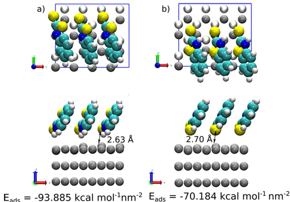
**Fig. 9** Top view and side view for the final adsorption structures at high concentration (3 molecules per  $\text{nm}^2$  obtained for 2-MBT on Zn(0001): a) (S,NH)-Zn, and b) (S,S)-Zn cases. White, cyan, yellow, blue, and gray colored spheres represent H, C, S, N, and Zn atoms, respectively. On the top view of each case, degraded color spheres represent the Zn under the surface.
