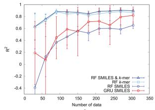
Fig. 9 Sample size dependence of  $R^2$  for four models: random forest and GRU with the modified-SMILES as an explanatory variable, random forest (RF) with supplementary values as explanatory variables, and random forest with the modified-SMILES and supplementary values as explanatory variables.
