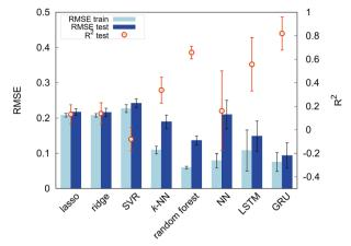
Fig. 6 Comparison of model performance using the modified-SMILES as explanatory variables, with both the RMSE and model coefficient of determination (R2) being shown. Error bars represent the standard deviation
