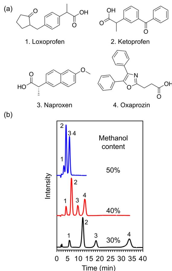
**Fig. 6** (a) Chemical structures of NSAIDs. (b) Chromatograms of mixed sample of four NSAIDs on ACCHexEE column. Analytical condition: mobile phase: 50 mM citrate buffer (pH 5)/methanol; column temperature: 25 °C; flow rate:  $0.2 \text{ mL min}^{-1}$ ; concentration:  $0.1 \text{ mg mL}^{-1}$ ,  $10 \mu\text{L}$  injection.
