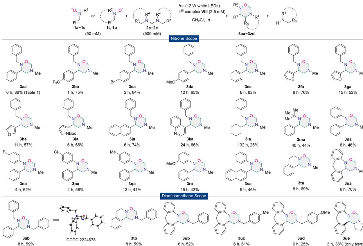
**Scheme 2** Scope of nitrones and *N,N,N',N'*-tetraalkyldiaminomethanes. Reaction conditions: nitronne **1** (50 mM), *N,N,N',N'*-tetraalkyldiaminomethane **2** (500 mM), and Ir<sup>III</sup> complex **VIII** (2.5 mM) in CH<sub>2</sub>Cl<sub>2</sub>, irradiated using the LED strip ( $\lambda = 400\text{--}780$  nm, 12 W, 60 white LEDs per m). All products were isolated.
