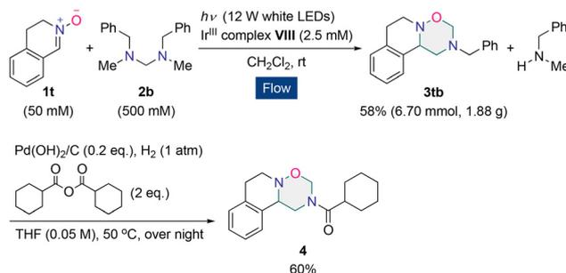
**Scheme 4** Gram-scale photoflow synthesis of **3tb** and preparation of **4**. LED tape length, 4 m (60 LEDs per m); PTFE tube O.D. 1.59 mm, I.D. 0.8 mm, 3.75 m; average flow rate  $0.0420 \text{ mL min}^{-1}$ ; total amount of liquid fed, 231 mL; residence time, 45 min.
