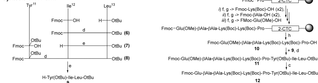
Scheme 1 Reagents and conditions: a) Fmoc-β-Ala-OH, HATU, DIPEA, DMF, 0 °C, then rt, on; b) methyl bromoacetate, K 2 CO 3 , ACN, rt, on; c) NaOH, CaCl 2 , i Pr-OH/H 2 O 7:3, rt, TLC monitoring; d) HATU, DMF, 0 °C, then rt, on; e) 20% piperidine in DMF, 1 h, rt; f) 20% piperidine in DMF, 5 min × 3, rt, in an SPPS syringe; g) HATU, DIPEA, appropriate Fmoc-AA-OH, 1 h, rt, in an SPPS syringe; h) DCM, TFE, AcOH (8:1:1), 4 h, rt, in an SPPS syringe. All reactions were performed in a round bottom flask unless otherwise specified.
