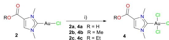
Scheme 4 Preparation of monocarbene gold(III) complexes 4a–c from monocarbene gold(I) complexes 2a–c . Reagents and reaction conditions: i) 1.4 eq. PhICl 2 , DCM or DCM/MeOH, 24 h, rt.
