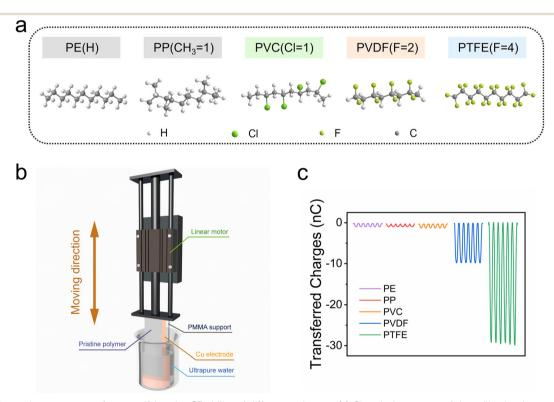
Fig. 1 Experimental measurement for quantifying the CE ability of different polymers. (a) Chemical structure of the utilized polymers. (b) Schematic illustration of the evaluation of the CE ability of the polymers using a single-electrode mode triboelectric nanogenerator (SE-TENG) that repeatedly comes into contact with DI water. (c) Quantity of charges transfer measured when the different polymers were used for CE with DI water.
