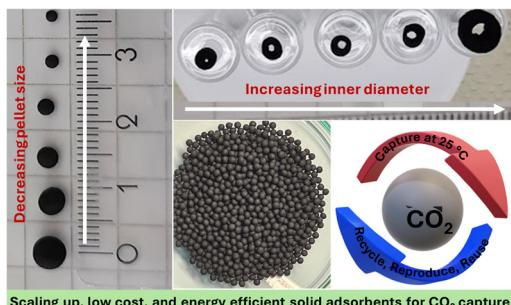
Porous carbon pellets for physical adsorption of CO<sub>2</sub>: size and shape effect
