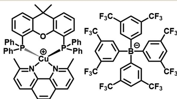
Fig. 1 Chemical structure of complex 1 with counterion  $\text{tfpb}^-$ . Structure of complex 1 obtained by single crystal X-ray crystallography, which is fully consistent with that published previously, is given in the ESI,† Fig. S8. CCDC 2012235.
