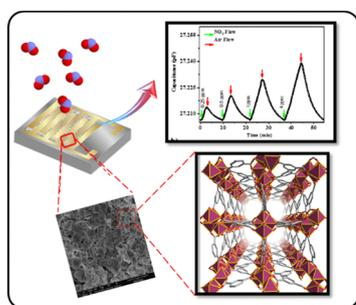
The deployment of an NOTT-300 (Al) MOF thin film as a NO<sub>2</sub> capacitive sensor under ambient conditions
