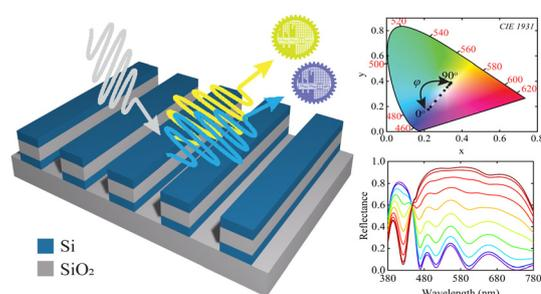
An ingenious Si-SiO<sub>2</sub>-Si grating dielectric metasurface structure was engineered to obtain structural colorization.
