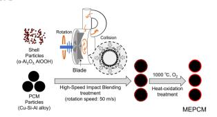
High-temperature ternary Cu-Si-Al alloy as a core-shell microencapsulated phase change material: fabrication via dry synthesis method and its thermal stability mechanism
