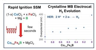
Rapid solid-state metathesis reactions for the formation of cobalt-iron monoboride solid-solutions and investigation of their water splitting electrocatalytic activity
