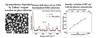
Arresting Tollens' reagent's reaction on a glass surface as the easiest method to fabricate Aq nanocluster-based SERS substrates for glucose sensing
