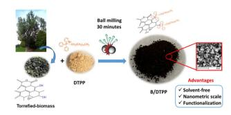
Eco-friendly one-shot approach for producing a functionalized nano-torrefied biomass: a new application of ball milling technology
