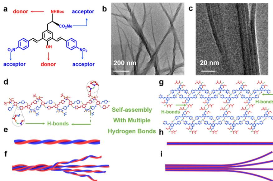
**Scheme 1** Illustration of the supramolecular self-assembly pathway (a) molecular structure of an *m*-phenylene vinylene (*m*-PPV) derivative compound **L2**, designed with hydrogen bonding donors and acceptors. Cryo-TEM images of (b) helical fibres and (c) straight self-assembled fibres assembled from compound **L2** in DMSO and DMSO/water mixture. Schematics depicting (d)–(f) the assembly of helical fibres, and (g)–(i) the formation of straight fibres through multiple hydrogen bonds.
