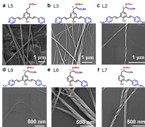
Fig. 3 SEM images showing the effect of the chiral centre. (a) Achiral bis-styryl-L-tyrosine analogue formed nanowires without helicity (straight nanowires). (b) Chiral bis-styryl-L-tyrosine analogue formed helical nanowires. (c)–(f) Self-assembled helical fibres resulting from chiral molecules with different functional groups on the end.
