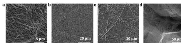
**Fig. 2** SEM images of large area of self-assembled fibre of compound **L2** in DMSO on different substrates: (a) Si (b) Al (c) ITO (d) graphite.
