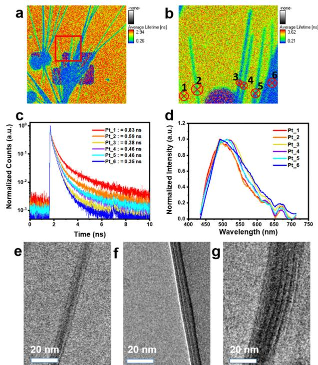
**Fig. 5** FLIM of the self-assemblies. (a) FLIM images of nanofibres. (b) Zoom out of the red box in (a). (c) Lifetime and (d) emission spectra of single nanofibres at points 1–6 labelled in (b). (e)–(g) Cryo-TEM images of **L2** revealing nanofibre bundles composed of parallel nanofibres with diameters of approximately 2–3 nm. As hypothesized, the h-bonding was formed in both x direction and y direction.
