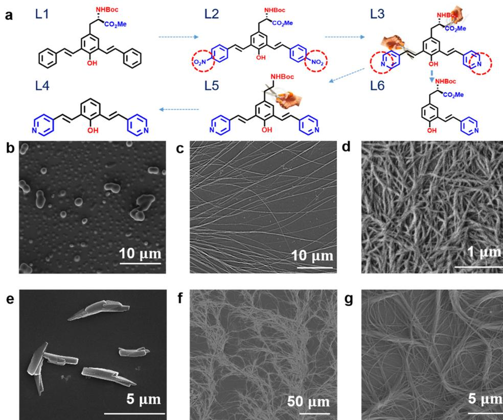
**Fig. 1** Schematic diagram and SEM images showing the relation between molecular structure and self-assembled morphology. (a) Molecular structures of tyrosine derivatives **L1**–**L6** with various functional groups. The change or removal of functional groups is indicated by circles and scissors, respectively. (b)–(g) SEM images of the self-assembled architectures formed by **L1**–**L6** on Si substrates, respectively.
