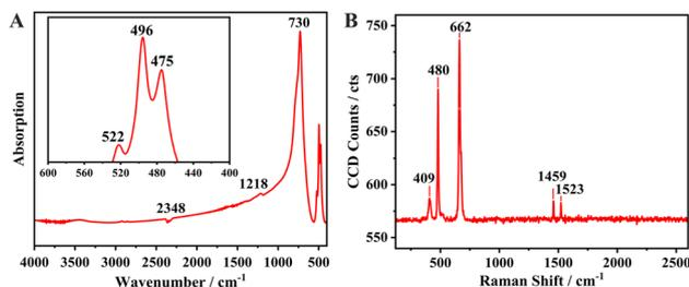
**Fig. 2** (A) Infrared spectrum of  $\text{Na}_6\text{Si}_3\text{F}_{18}$ . (B) Single-crystal Raman spectrum of  $P321$  phase  $\text{Na}_6\text{Si}_3\text{F}_{18}$  in the range of  $120\text{--}2600\text{ cm}^{-1}$ .
