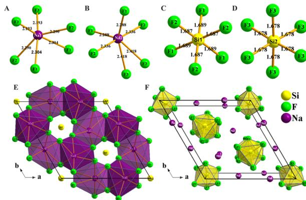
**Fig. 1** Crystal structure of  $\text{Na}_6\text{Si}_3\text{F}_{18}$ . (A) Coordination of the Na1 atom; (B) coordination of the Na2 atom; (C) coordination of the Si1 atom; (D) coordination of the Si2 atom; (E) parallel projection of the corner-linked  $[\text{NaF}_6]$  octahedron structure viewed down  $[111]$ ; (F) central projection of isolated  $[\text{SiF}_6]$  octahedron viewed down  $[111]$  in the primitive cell.
