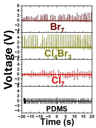
Fig. 6 Piezoelectric properties of the perovskite/PDMS composite films: output voltage of PDMS (black),  $Cl_7/PDMS$  (red),  $Cl_4Br_3/PDMS$  (yellow), and  $Br_7/PDMS$  (dark red) composite films under a periodic pressuring and releasing process with a knocking pen.
