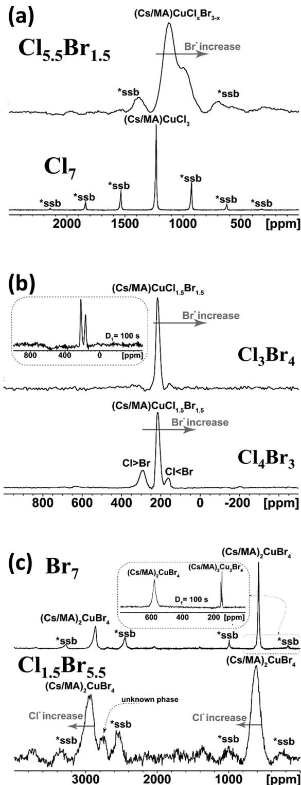
Fig. 3 Experimental  $^{133}\text{Cs}$  VF/MAS NMR spectra of (a)  $\text{Cl}_7$ ,  $\text{Cl}_{5.5}\text{Br}_{1.5}$ , (b)  $\text{Cl}_4\text{Br}_3$ ,  $\text{Cl}_3\text{Br}_4$ , and (c)  $\text{Cl}_{1.5}\text{Br}_{5.5}$ ,  $\text{Br}_7$ , respectively. The asterisks (\*ssb) denote spinning sidebands.
