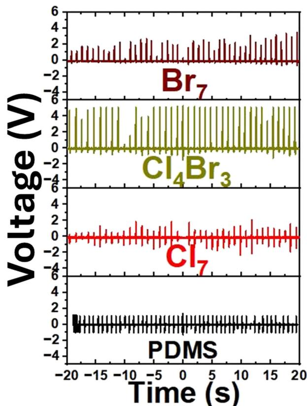
Fig. 6 Piezoelectric properties of the perovskite/PDMS composite films: output voltage of PDMS (black),  $\text{Cl}_7$ /PDMS (red),  $\text{Cl}_4\text{Br}_3$ /PDMS (yellow), and  $\text{Br}_7$ /PDMS (dark red) composite films under a periodic pressing and releasing process with a knocking pen.
