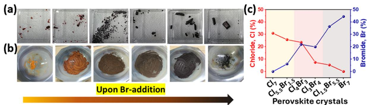
Fig. 1 Copper perovskite crystals prepared *via* the slow evaporation method (a) and after grinding with mortar and pestle (b) where the samples from left to right are: Cl<sub>7</sub>, Cl<sub>5.5</sub>Br<sub>1.5</sub>, Cl<sub>4</sub>Br<sub>3</sub>, Cl<sub>3</sub>Br<sub>4</sub>, Cl<sub>1.5</sub>Br<sub>5.5</sub>, and Br<sub>7</sub>, respectively. (c) Data from energy dispersive spectroscopy (EDS) for determining the (Cl/Br) content of perovskite crystals.
