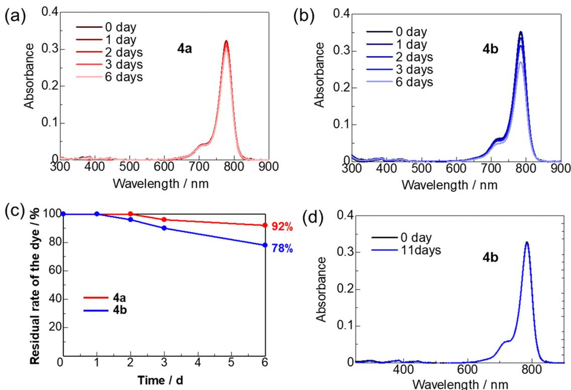
Fig. 9 Photostabilities of HMCDs **4a** and **4b** under white LED irradiation (8.5 W) in an incubator at 25 °C in  $CH_2Cl_2$  solutions ( $1 \times 10^{-6}$  M).
