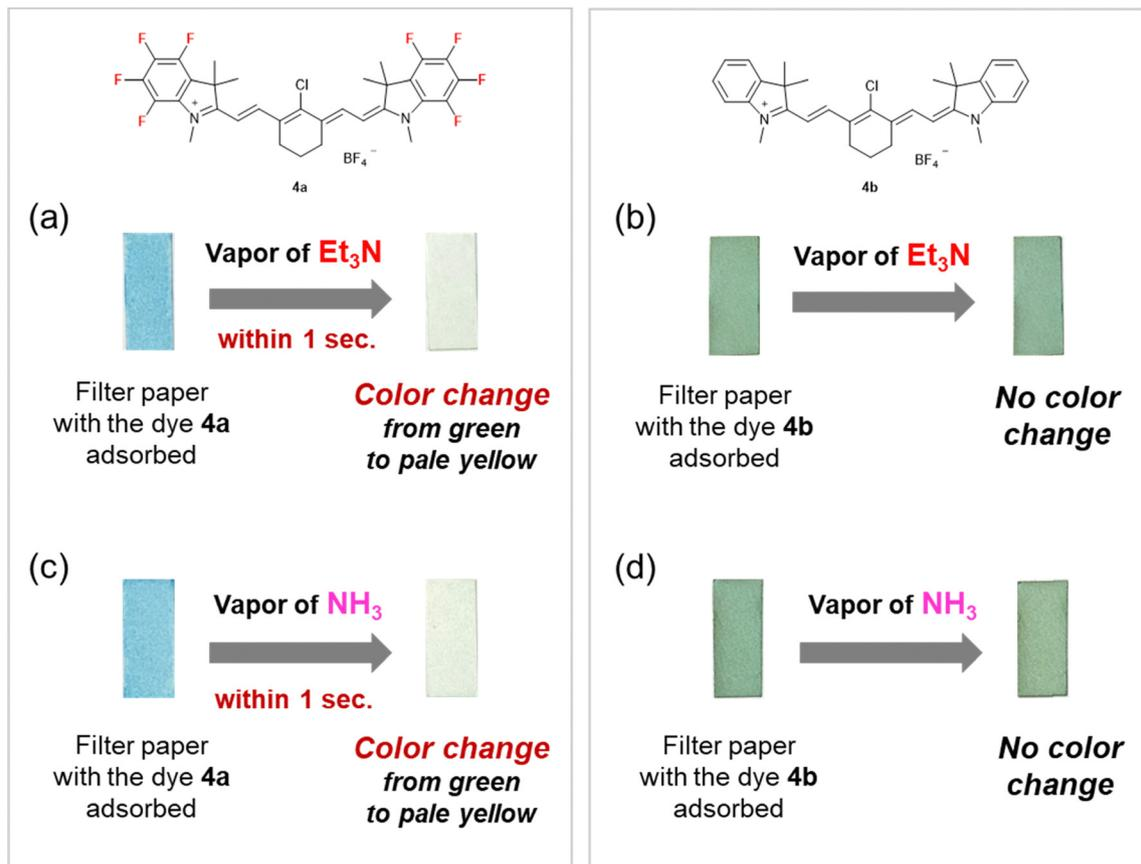
Fig. 12 Photographs of ring-fluorinated HMCD **4a** adsorbed on the filter paper with TEA vapour (a), HMCD **4b** adsorbed on the filter paper with TEA vapour (b), ring-fluorinated HMCD **4a** adsorbed on the filter paper with  $\text{NH}_3$  vapour (c), and HMCD **4b** adsorbed on the filter paper with  $\text{NH}_3$  vapour (d).
