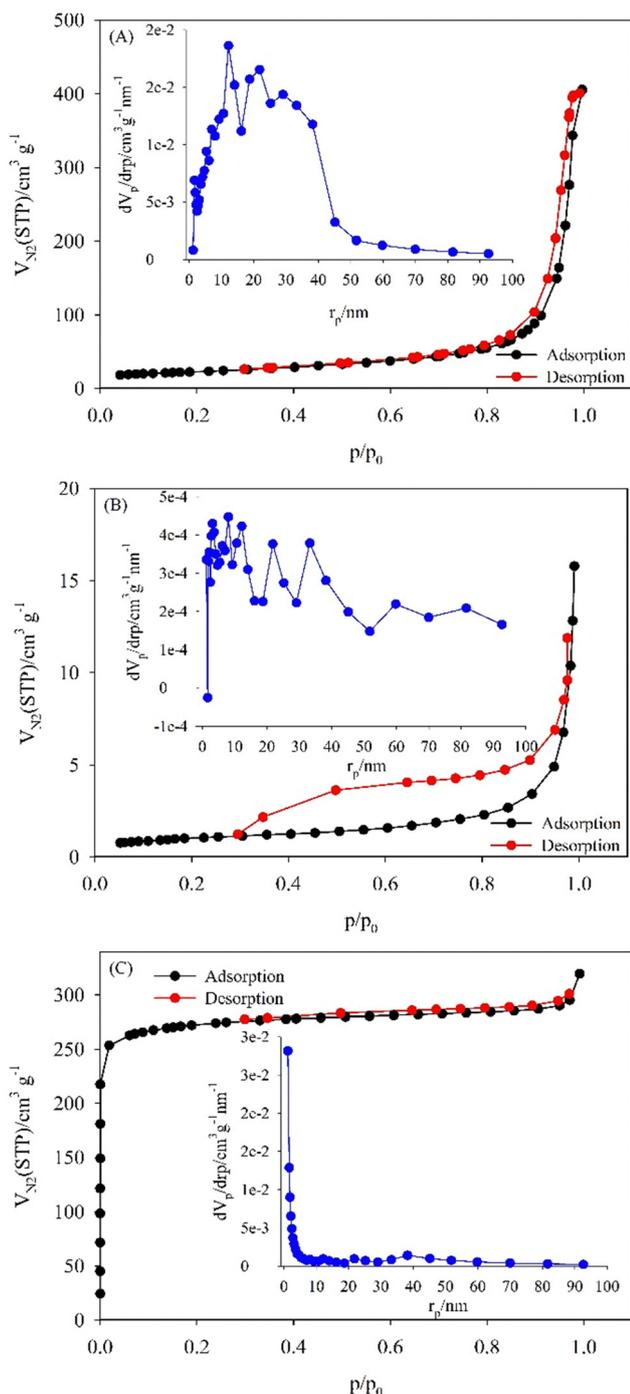
Fig. 3 Nitrogen adsorption–desorption BET isotherms of (A) Cu–BTC, (B) SiW<sub>11</sub>Co@Cu–BTC, and (C) SiW<sub>11</sub>Co@Cu–BTC/MWCNTs–COOH. The insets show the BJH-adsorption pore size distributions.
