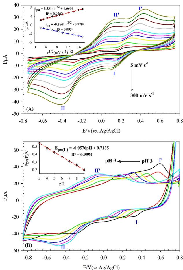
Fig. 7 (A) CVs of SiW<sub>11</sub>Co@Cu-BTC/MWCNTs-COOH/GCE in 0.04 M BRB (pH 7) in the presence of 0.5 mM DA at different scan rates from 5 to 300 mV s<sup>-1</sup>. The inset shows variations of the anodic and cathodic peak currents (peaks I, I') with scan rate. (B) In the presence of 200  $\mu\text{M}$  DA at different pHs (pH 3–9); scan rate 50 mV s<sup>-1</sup>. The inset shows the variation of the anodic peak potentials ( $E_{\text{pa}}$ ) with pH.
