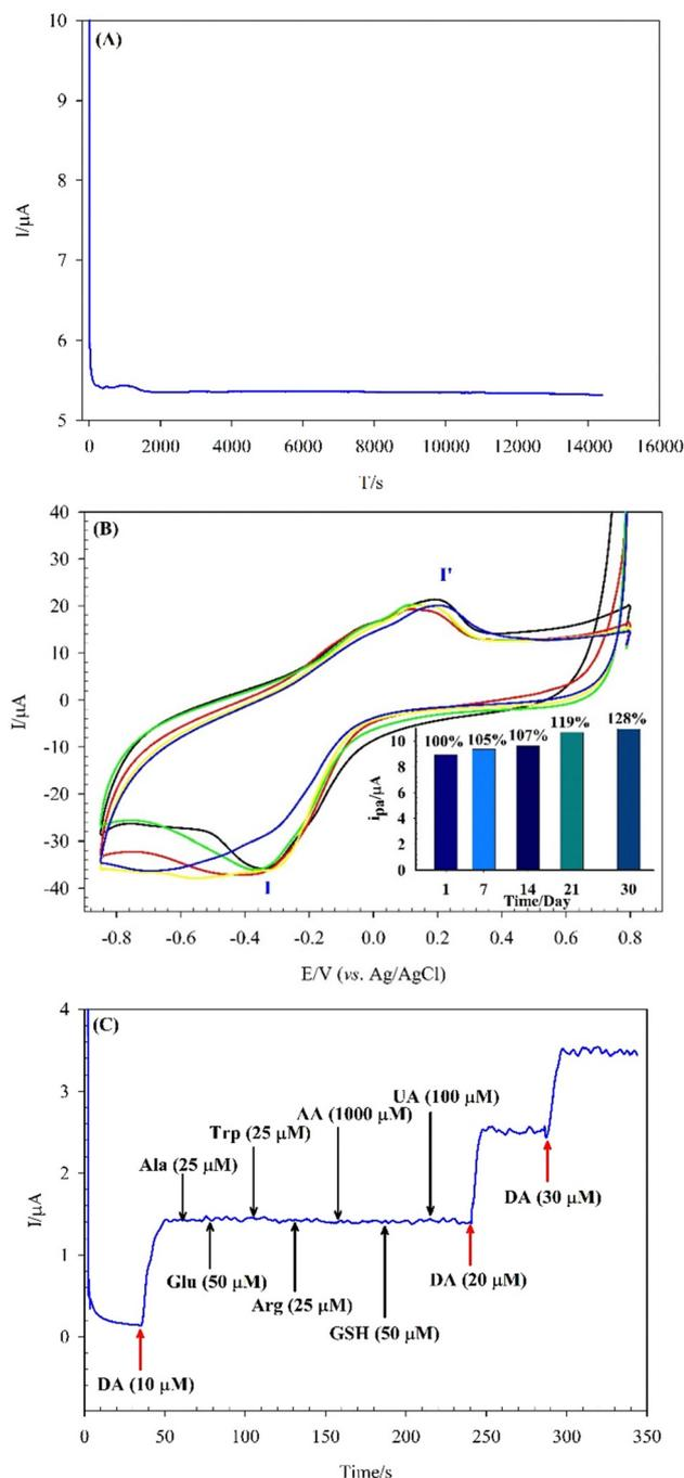
**Fig. 8** (A) Stability of SiW<sub>11</sub>Co@Cu-BTC/MWCNTs-COOH/GCE in 0.04 M BRB (pH 7) containing 100  $\mu$ M DA by chronoamperometry ( $I-t$ ) at the fixed-potential of +0.25 V, (B) long-term stability of SiW<sub>11</sub>Co@Cu-BTC/MWCNTs-COOH/GCE in 0.04 M BRB (pH 7) during 30 days, and (C) effect of interfering species on the detection of DA at a potential of +0.25 V at SiW<sub>11</sub>Co@Cu-BTC/MWCNTs-COOH/GCE in 0.04 M BRB (pH 7).
