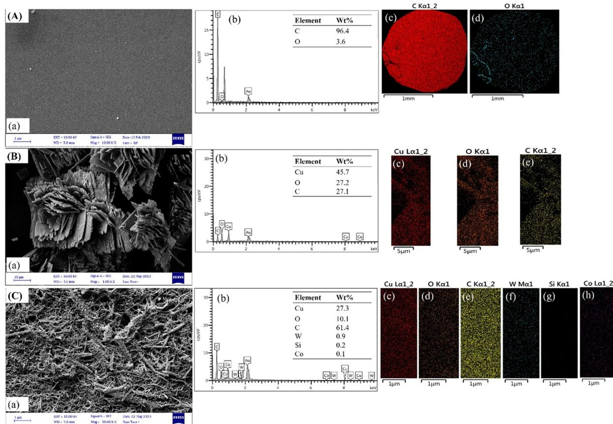
Fig. 4 FE-SEM images, EDX pattern, and EDX element mapping of the (A) bare GCE, (B) Cu-BTC/GCE, and (C) SiW<sub>11</sub>Co@Cu-BTC/MWCNTs-COOH/GCE.
