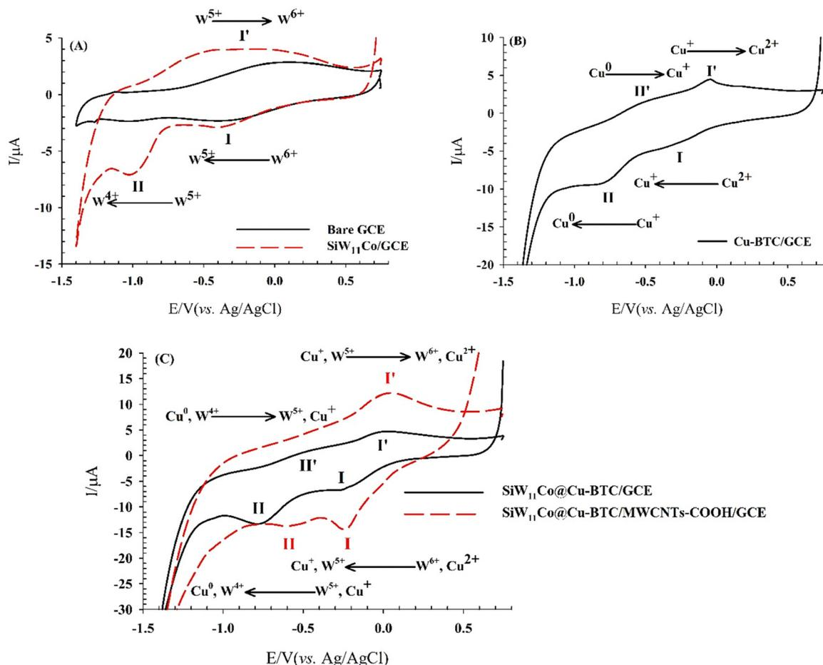
Fig. 5 CVs obtained on (A) bare GCE, and SiW<sub>11</sub>Co/GCE, (B) Cu-BTC/GCE, and (C) SiW<sub>11</sub>Co@Cu-BTC/GCE, and SiW<sub>11</sub>Co@Cu-BTC/MWCNTs-COOH/GCE in 0.04 M BRB (pH 7) and scan rate of 50 mV s<sup>-1</sup>.
