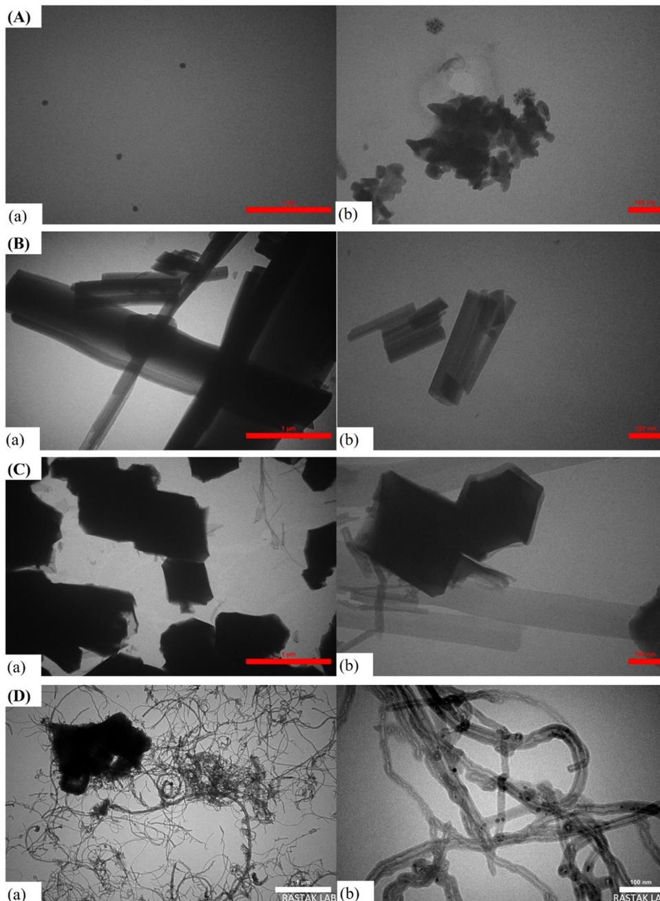
Fig. 2 TEM images of (A)  $\text{SiW}_{11}\text{Co}$  (a) and (b), (B)  $\text{Cu-BTC}$  (a) and (b), (C)  $\text{SiW}_{11}\text{Co@Cu-BTC}$  (a) and (b), and (D)  $\text{SiW}_{11}\text{Co@Cu-BTC/MWCNTs-COOH}$  (a) and (b) at different magnifications.
