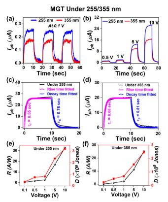
Fig. 6 MGT: transient (I-t) photo response curve under 255 and 355 nm laser illuminations at (a) 0.1 V and (b) 0.5-10 V. (c) and (d) Fitted time response curves and (e) and (f) responsivity and detectivity versus voltage graphs of MGT under 255 and 355 nm laser illuminations, respectively.
