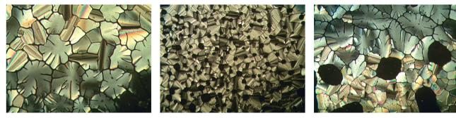
Fig. 2 Polarized light photomicrographs of the columnar mesophase of compounds 2 (T = 246 °C, left), 6 (T = 216 °C, middle) and 7 (T = 185 °C right) all taken on cooling
