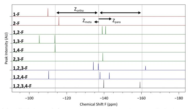
Fig. 5 Stacked 19F NMRs of compounds 1 to 9, arranged with increasing number of fluorine atoms from top to bottom. The effect of substituents at various positions (ortho, meta and para) are shown, along with a reference line (dashed) showing the effect of one or two ortho substituents on the compounds
