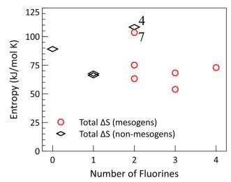
**Fig. 4** Transition entropy for compounds **1–10**, arranged as in Fig. 3. Entropies are calculated as the transition enthalpies (taken on heating) divided by the transition temperatures. For the mesogens, the entropies of each transition have been added together for comparison with the non-mesogens.
