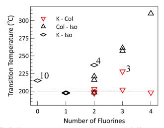
Fig. 3 Phase transition temperatures for compounds 1-10, grouped based on the extent of fluorination. Plot markers show the transition temperatures on heating (see Table 1). The isotropic transition tends to increase in temperature with fluorination, while the crystal transition is nearly constant across the different compounds (the dotted line is a guide for the eye).
