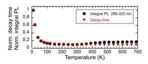
Fig. 9 Temperature dependence of a normalised integral of PL spectra in the range of 295-325 nm excited with 275 nm and normalised PL decay time (exc. 275 nm, em. 312 nm), both norm. at 9 K.
