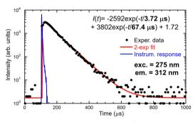
Fig. 7 Decay curve of 312 nm emission of Gd<sup>3+</sup>, the measured data are the convolution of IRF and decay equation in the figure.
