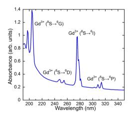
Fig. 4 Absorption spectrum of (Gd,Y)AlO<sub>3</sub>
