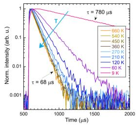
Fig. 10 Decay curves of the intrinsic Gd<sup>3+</sup> emission 312 nm as a function of temperature; the sample was excited at 275 nm
