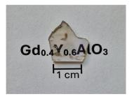
Fig. 2 Photograph of the (Gd,Y)AlO<sub>3</sub> sample.
