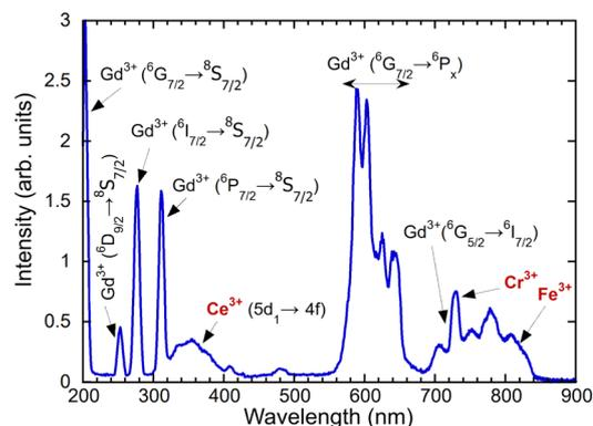
Fig. 5 Radioluminescence spectrum of  $(\text{Gd},\text{Y})\text{AlO}_3$ , X-ray excitation, 40 kV, 15 mA.
