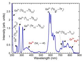
Fig. 5 Radioluminescence spectrum of (Gd,Y)AlO<sub>3</sub>, X-ray excitation, 40 kV, 15 mA
