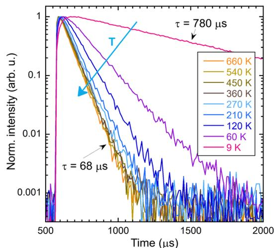
Fig. 10 Decay curves of the intrinsic Gd<sup>3+</sup> emission 312 nm as a function of temperature; the sample was excited at 275 nm.
