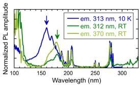
Fig. 8 Excitation spectra measured for different emission wavelengths (313 and 370 nm) and temperature 10 K and RT. Measured at the PETRA III
