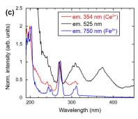
Fig. 6 (a) Emission spectra, excitation wavelengths 271, 310 and 370 nm; (b) excitation spectra, emission wavelengths 312, 589 and 725 nm; (c) excitation spectra, emission wavelengths 354, 525 and 750 nm.
