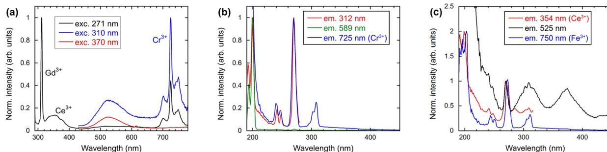
Fig. 6 (a) Emission spectra, excitation wavelengths 271, 310 and 370 nm; (b) excitation spectra, emission wavelengths 312, 589 and 725 nm; (c) excitation spectra, emission wavelengths 354, 525 and 750 nm.
