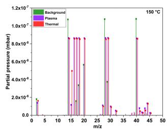
Fig. 3 Bar scan spectra showing the background (green) with no precursor, co-reactant or plasma power turned on and detected masses during ALD cycles when TDMAA and NH3 were pulsed at 150 °C for the plasma (violet) and thermal (red) processes. Small mass offsets in m/zvalues on the horizontal axis were introduced for visual clarity
