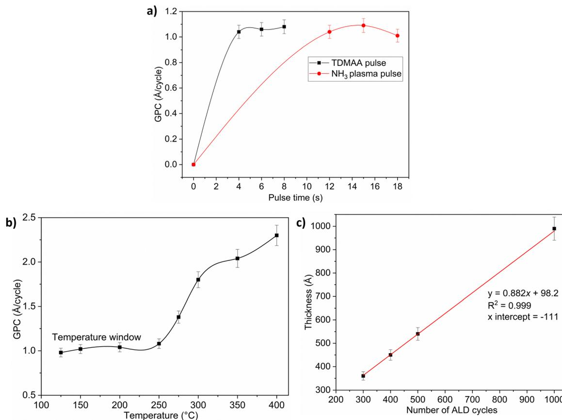
Fig. 1 Saturation curves for the plasma process, showing the effect of the TDMAA pulse time and the NH<sub>3</sub> plasma pulse time on the GPC (a). The plasma process growth dependence on process temperature is shown in (b) while film thickness dependence on number of cycles, showing no nucleation delay, for the plasma process is illustrated in (c).
