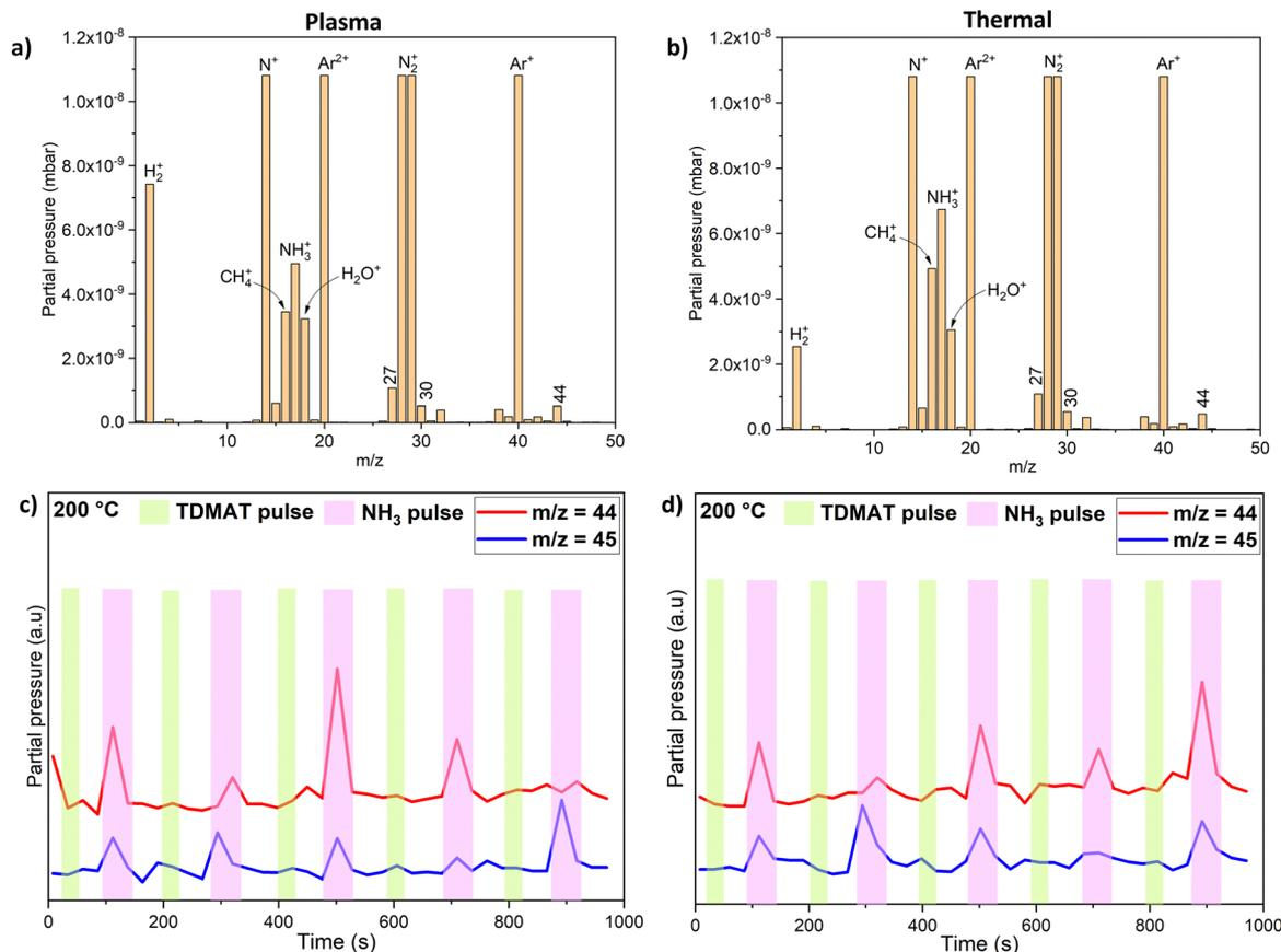
Fig. 7 Bar scan spectra showing detected masses during ALD cycles when TDMAT and NH<sub>3</sub> are pulsed at 200 °C during a plasma process (a) and a thermal process (b). Mass spectrometric time behaviour of detected N(CH<sub>3</sub>)<sub>2</sub> (*m/z* = 44) and HN(CH<sub>3</sub>)<sub>2</sub> (*m/z* = 45) during TiN growth from TDMAT and NH<sub>3</sub> at 200 °C for a plasma process is displayed in (c) while the thermal process is displayed in (d).
