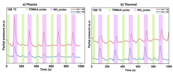
Fig. 4 Main reaction products (m/z = 44 and m/z = 45) created during the plasma (a) and thermal (b) processes at 150 °C probed and monitored over time by the mass spectrometer
