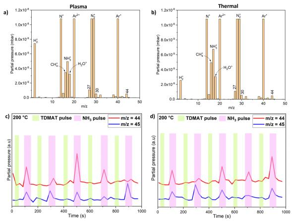
Fig. 7 Bar scan spectra showing detected masses during ALD cycles when TDMAT and NH<sub>3</sub> are pulsed at 200 °C during a plasma process (a) and a thermal process (b). Mass spectrometric time behaviour of detected N(CH<sub>3</sub>)<sub>2</sub> (m/z = 44) and HN(CH<sub>3</sub>)<sub>2</sub> (m/z = 45) during TiN growth from TDMAT and  $NH_3$  at 200 °C for a plasma process is displayed in (c) while the thermal process is displayed in (d).
