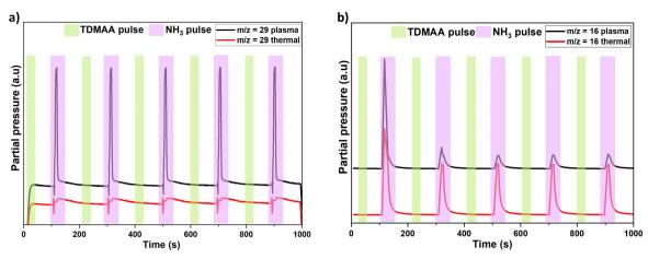
Fig. 5 Mass spectrometric time behaviour of other detected species m/z = 29 (a) and m/z = 16 (b), during five AlN growth cycles in plasma and thermal processes.
