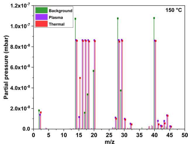
Fig. 3 Bar scan spectra showing the background (green) with no precursor, co-reactant or plasma power turned on and detected masses during ALD cycles when TDMAA and  $\text{NH}_3$  were pulsed at 150 °C for the plasma (violet) and thermal (red) processes. Small mass offsets in  $m/z$  values on the horizontal axis were introduced for visual clarity.
