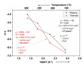
Fig. 9 Arrhenius plot for NH<sub>3</sub> reaction on a TDMAA-terminated surface, emitting dimethylamine, in plasma (black line) and thermal (red line) processes, during the NH<sub>3</sub> pulse. Straight lines (not shown) represent a weighted linear fit to the data, from which the corresponding Arrhenius parameters were drawn.
