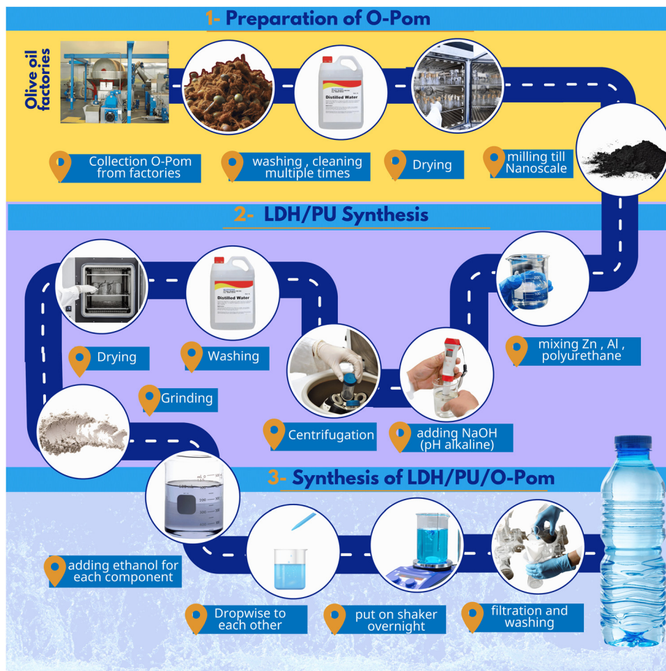
Scheme 1 Schematic illustration of the applied material preparation.
