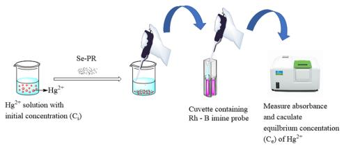
Fig. 7 Protocol for the quantitative determination of Hg<sup>2+</sup> ions using colorimetry.
