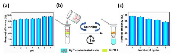
Fig. 9 (a) Effect of pH on the adsorption capacity, (b) spin column treatment of contaminated water and (c) recyclability test for Se-PR  $\mathbf{2}$ , with an initial Hg<sup>2+</sup> ion concentration of 1.5 mM (300 mg L<sup>-1</sup>).
