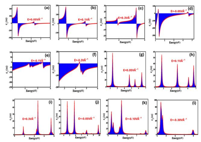
Fig. 8 Electric-field mediated engineering and modulation of the (a)–(f) real  $(\varepsilon_1(\omega))$  part of dielectric (g)–(l) imaginary  $(\varepsilon_2(\omega))$  part of dielectric function of zinc blende ZnSe compounds calculated by GGA process.
