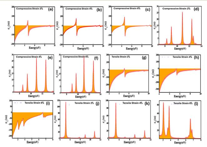
Fig. 9 (a-l) Biaxial compressive and tensile strain mediated engineering and modulation of the real  $(\varepsilon_1(\omega))$  and imaginary  $(\varepsilon_2(\omega))$  part of dielectric function of zinc blende ZnSe compounds calculated by GGA process.
