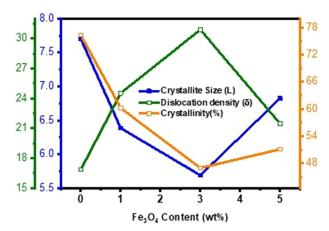
Fig. 4 Variation of crystallite size (L), dislocation density ( $\delta$ ) and % crystallinity ( $\psi$ ) of pure  $\delta$ -MnO<sub>2</sub> nanoflower and  $\delta$ -MnO<sub>2</sub>/Fe<sub>3</sub>O<sub>4</sub> nanocomposites obtained from XRD line profile analysis as function of Fe<sub>3</sub>O<sub>4</sub> content. The 3% incorporation of Fe<sub>3</sub>O<sub>4</sub> nanodiamonds results in the highest dislocation density, smallest crystallite size and lowest % of crystallinity
