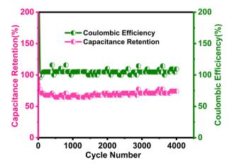
Fig. 11 Long term cyclic stability performance as capacitive retention and Coulombic efficiency of the  $\delta$ -MnO<sub>2</sub>/(3%) Fe<sub>3</sub>O<sub>4</sub> nanocomposite sample at  $6 \text{ A g}^{-1}$  current density over 4000 cycles of operation.
