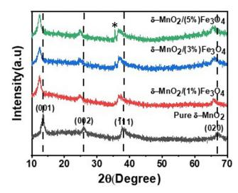
Fig. 3 XRD patterns of pure  $\delta$ -MnO<sub>2</sub> nanoflower and  $\delta$ -MnO<sub>2</sub>/Fe<sub>3</sub>O<sub>4</sub> nanocomposites. The asterisk corresponds to (311) peak from Fe<sub>3</sub>O<sub>4</sub> nanodiamond and its intensity increases with increase in Fe<sub>3</sub>O<sub>4</sub> content.
