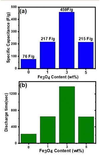
Fig. 9 (a) Specific capacitance of the samples as a function of Fe $_3$ O $_4$  content, the  $\delta$ -MnO $_2$ /(3%) Fe $_3$ O $_4$  nanocomposite shows the highest specific capacitance; (b) discharge time of the samples as a function of Fe $_3$ O $_4$  content, obtained from the GCD curves in Fig. 8(a).
