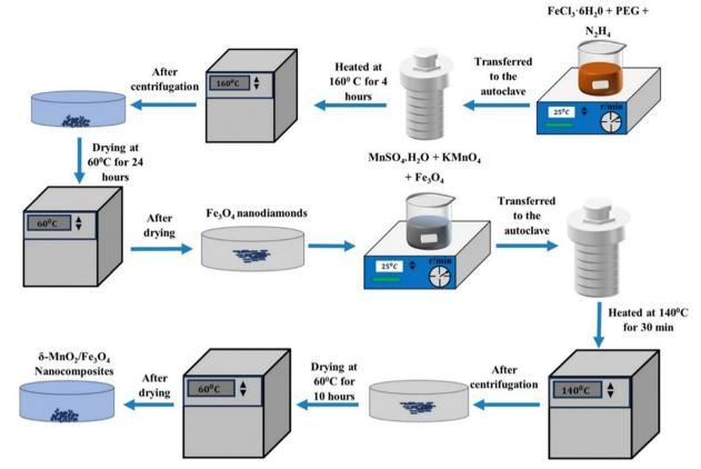
Fig. 1 Flowchart showing  $\delta$ -MnO<sub>2</sub>/Fe<sub>3</sub>O<sub>4</sub> nanocomposite synthesis process. After synthesizing Fe<sub>3</sub>O<sub>4</sub> nanodiamonds, it is mixed into the precursor solution of  $\delta$ -MnO<sub>2</sub> nanoflowers at 1, 3 and 5 wt% producing  $\delta$ -MnO<sub>2</sub>/(1%) Fe<sub>3</sub>O<sub>4</sub>,  $\delta$ -MnO<sub>2</sub>/(3%) Fe<sub>3</sub>O<sub>4</sub> and  $\delta$ -MnO<sub>2</sub>/(5%) Fe<sub>3</sub>O<sub>4</sub> nanocomposites, respectively.
