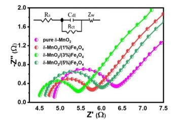
Fig. 10 EIS spectra of as-prepared pure  $\delta$ -MnO<sub>2</sub> nanoflowers and  $\delta$ -MnO<sub>2</sub>/Fe<sub>3</sub>O<sub>4</sub> nanocomposite electrodes. The inset shows equivalent Randle's circuit. Different electrical components of this circuit were obtained from fitting the experimental EIS spectra with Randle's circuit *via* Z View software.
