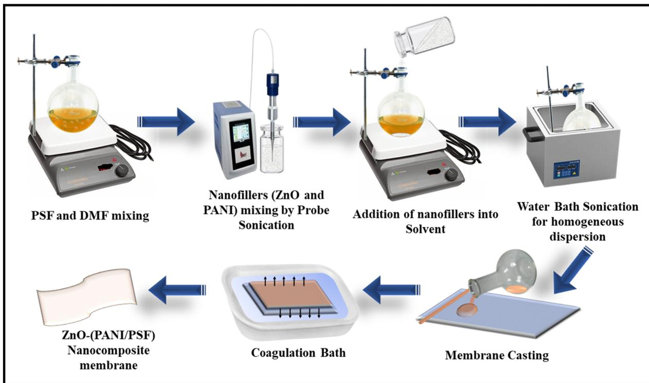
Fig. 1 Fabrication of ZnO-(PANI/PSF) composite membranes by phase inversion.
