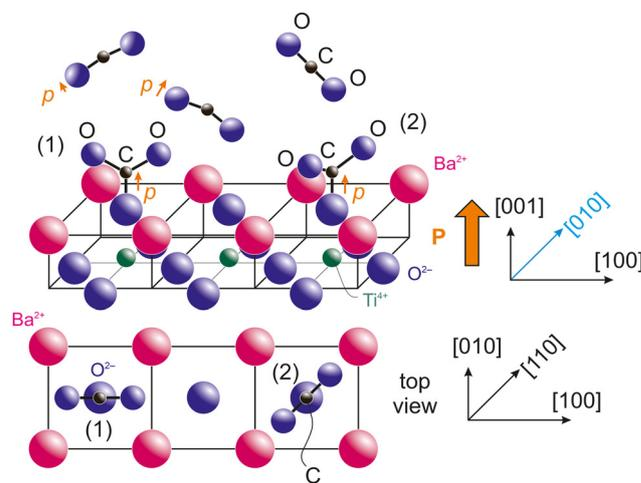
**Fig. 7** Proposal for adsorption geometries with  $\text{CO}_2$  bound to a surface oxygen, with two possible azimuthal orientation of the  $\text{CO}_3$  plane: (1) along the in-plane [100] axis and (2) along the in-plane [110] axis. The top drawing is a perspective view, and the bottom drawing a top view. Electrostatic evaluation of the interaction of terminal oxygens with surface  $\text{Ba}^{2+}$  cations suggest that the geometry (2) is slightly favored.
