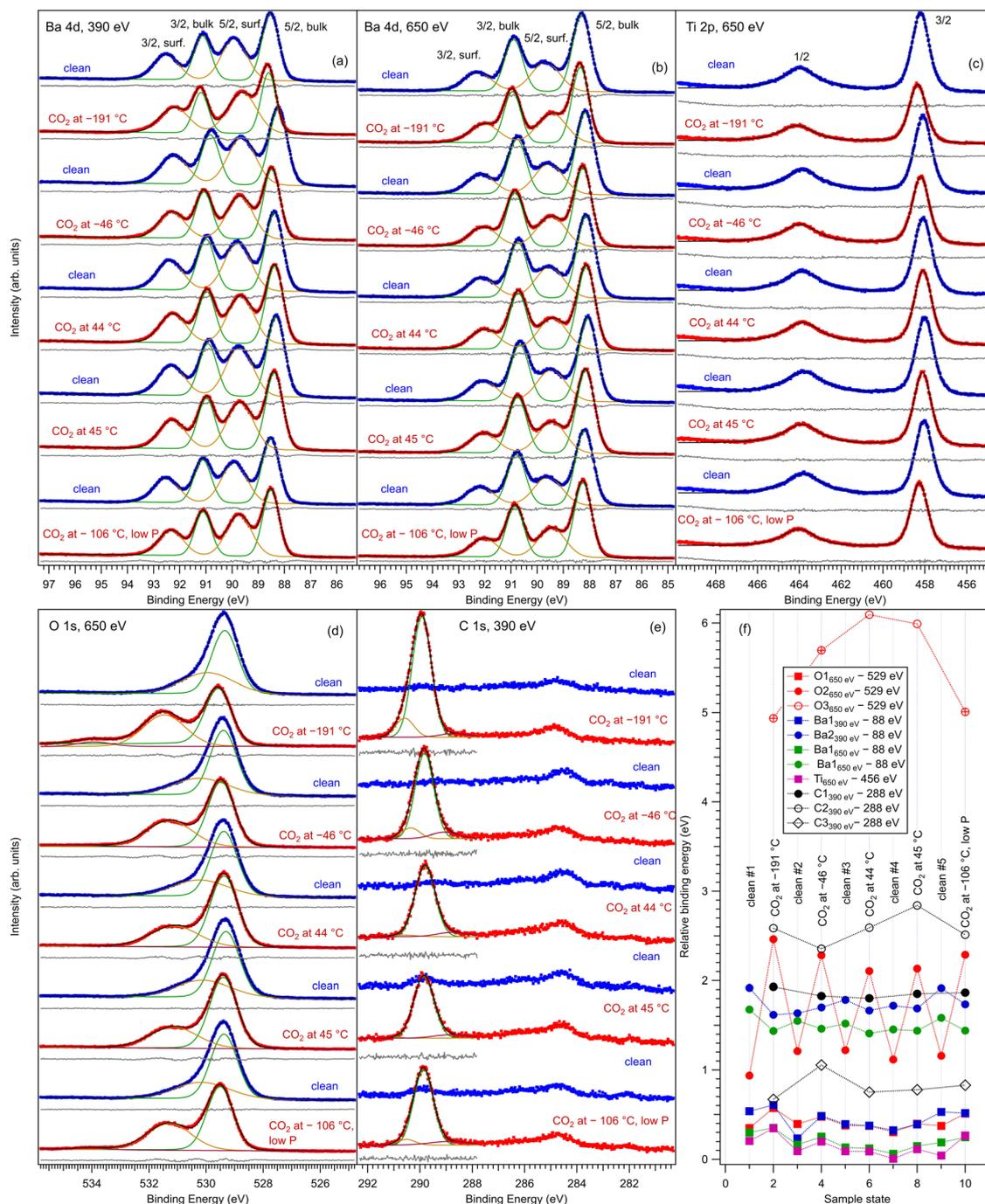
Fig. 2 Core level X-ray photoelectron spectroscopy for Ba 4d (a) and (b), Ti 2p (c), O 1s (d) and C 1s (e) for BaTiO<sub>3</sub>(001) clean and after several doses with 3.4 kL CO<sub>2</sub> at different temperatures. The employed photon energies are specified on each graph. (f) Represents the variation in extracted binding energies from the analysis of the spectra for each surface state.
