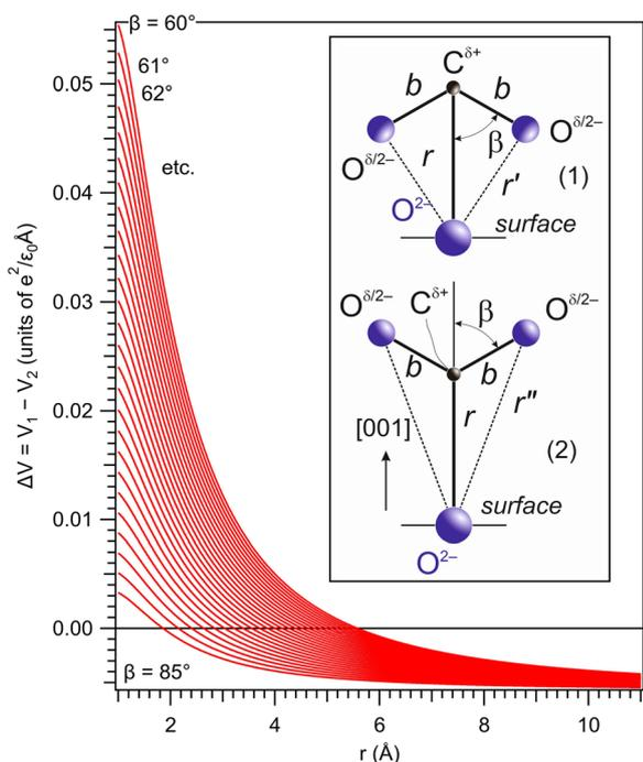
**Fig. 8** The potential energy difference between the configuration with the oxygens from the bent  $\text{CO}_2$  oriented towards the BTO(001) surface and that with the carbon closer to the BTO(001) surface. When this energy difference is positive, the molecule is supposed to be oriented with the carbon towards a surface oxygen anion.
