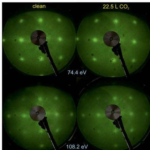
Fig. 1 Low energy electron diffraction (LEED) images on clean  $\text{BaTiO}_3(001)$  and after  $\text{CO}_2$  dosing (22.5 L). The electron energies are indicated on the figure.
