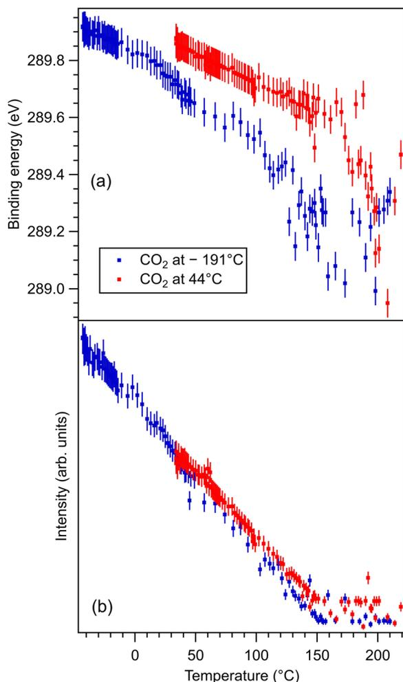
**Fig. 6** (a) Extracted temperature variations of the binding energy for C 1s spectra; (b) extracted temperature variation of the integral amplitude, with the same color code as in (a). The spectra and their peak fitting analyses are presented in Fig. S12 and S13 (ESI†).
