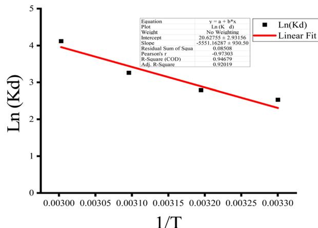
Fig. 15 Sorption thermodynamic parameters of MB dye sorption on the nZVI-TiO<sub>2</sub>-SiO<sub>2</sub> nanocomposite.
