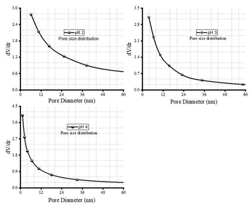
Fig. 5 Pore size distribution curves of the SiO<sub>2</sub>-TiO<sub>2</sub>-nZVI nanocomposite synthesized at pH 2, 3 and 4.
