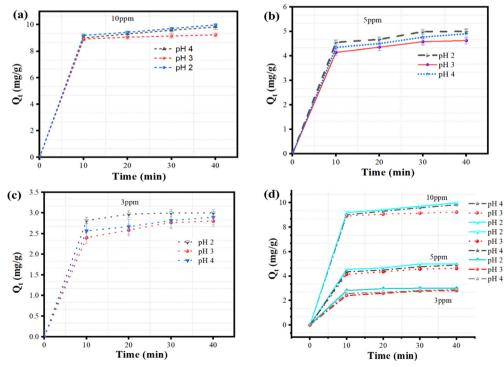
Fig. 10 Amount (mg  $g^{-1}$ ) of MB dye adsorbed per unit mass of nZVI-SiO<sub>2</sub>-TiO<sub>2</sub> at a given time, t (min). (a)–(c) The amount of MB dye adsorbed at a given time for  $C_0 = 10$  ppm,  $C_0 = 5$  ppm and  $C_0 = 3$  ppm; (d) comparison of the quantity adsorbed at different dye concentrations.
