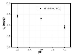
Fig. 13 Influence of synthesis pH on the equilibrium adsorption,  $q_e$  (mg q<sup>-1</sup>), of SiO<sub>2</sub>-TiO<sub>2</sub>-nZVI nanocomposites.
