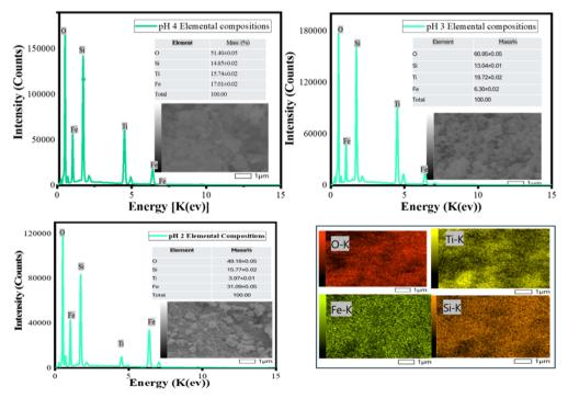
Fig. 3 Energy dispersive X-ray spectroscopy (EDS) of nZVI-SiO<sub>2</sub>-TiO<sub>2</sub> synthesized at pH 4, pH 3 and pH 2.
