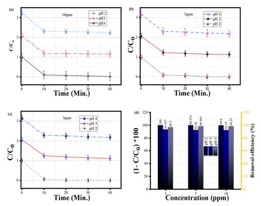
Fig. 9 Performance of the nZVI-SiO<sub>2</sub>-TiO<sub>2</sub> nanocomposite in the degradation and removal of methylene blue dye at different methylene blue dye concentrations: (a) 10 ppm methylene blue dye concentration, (b) 5 ppm methylene blue dye concentration and (c) 3 ppm methylene blue dye concentration. (d) Dye removal efficiencies versus concentrations.
