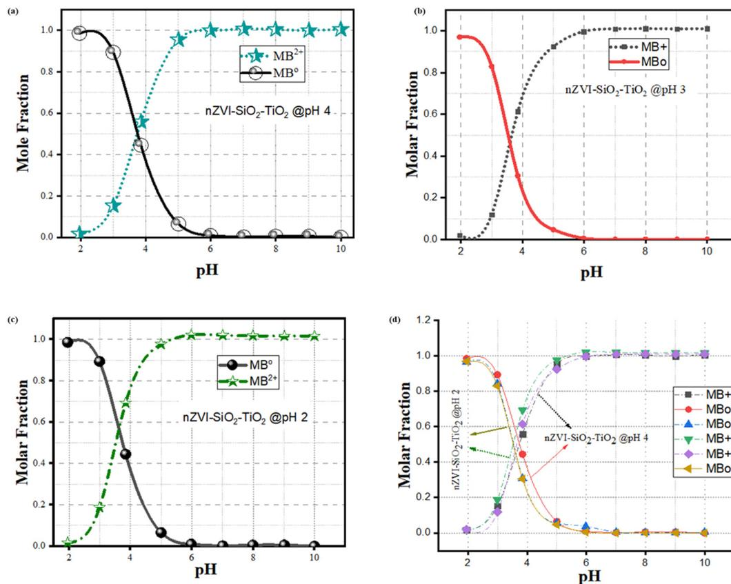
Fig. 17 Speciation behaviour of methylene blue dye following  $\text{SiO}_2\text{-TiO}_2\text{-nZVI}$  interaction under varying pH conditions: (a) pH 2, (b) pH 3, (c) pH 4, and (d) combined variable pH conditions, with an initial concentration of  $C_0 = 10 \text{ g L}^{-1}$ .
