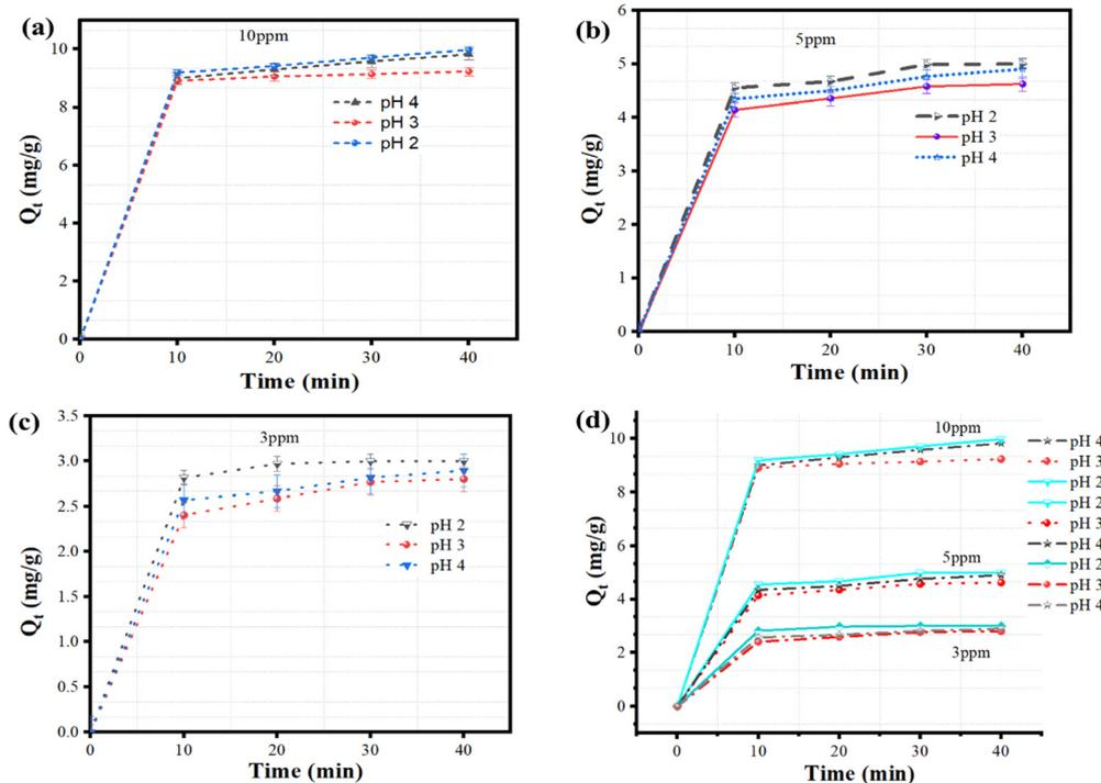
Fig. 10 Amount ( $\text{mg g}^{-1}$ ) of MB dye adsorbed per unit mass of nZVI-SiO<sub>2</sub>-TiO<sub>2</sub> at a given time,  $t$  (min). (a)-(c) The amount of MB dye adsorbed at a given time for  $C_0 = 10$  ppm,  $C_0 = 5$  ppm and  $C_0 = 3$  ppm; (d) comparison of the quantity adsorbed at different dye concentrations.
