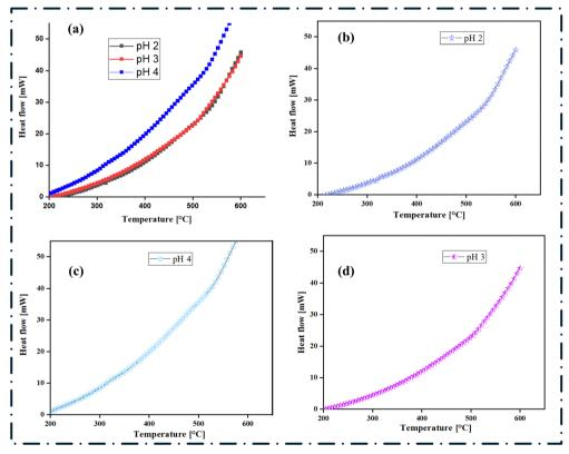
Fig. 7 Differential scanning calorimetry (DSC) analysis of SiO<sub>2</sub>-TiO<sub>2</sub>-nZVI nanocomposites synthesized under different pH conditions. (a) Stacked comparison of the thermal behaviour of SiO2-TiO2-nZVI under all three reaction conditions; (b) thermal behaviour of SiO2-TiO2-nZVI at pH 2; (c) thermal behaviour of SiO2-TiO2-nZVI at pH 3 and (d) thermal behaviour of SiO2-TiO2-nZVI at pH 4.
