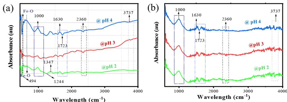
Fig. 14 FTIR spectra of the nZVI-SiO<sub>2</sub>-TiO<sub>2</sub> nanocomposites before (a) and after (b) MB dye degradation.
