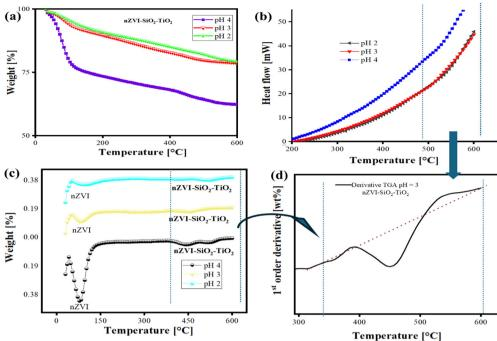
Fig. 8 Thermogravimetric analysis (TGA) and comparison of the thermal properties and characteristics of  $nZVI-SiO_2-TiO_2$  nanocomposites. (a) Stacked TGA plots, (b) stacked DSC plots and (c) and (d) TGA weight percent derivatives.
