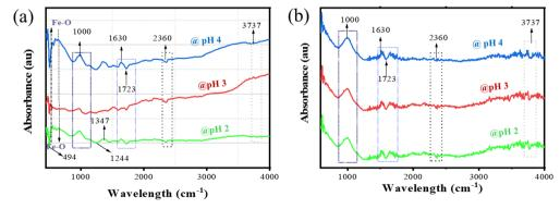
Fig. 14 FTIR spectra of the nZVI-SiO<sub>2</sub>-TiO<sub>2</sub> nanocomposites before (a) and after (b) MB dye degradation
