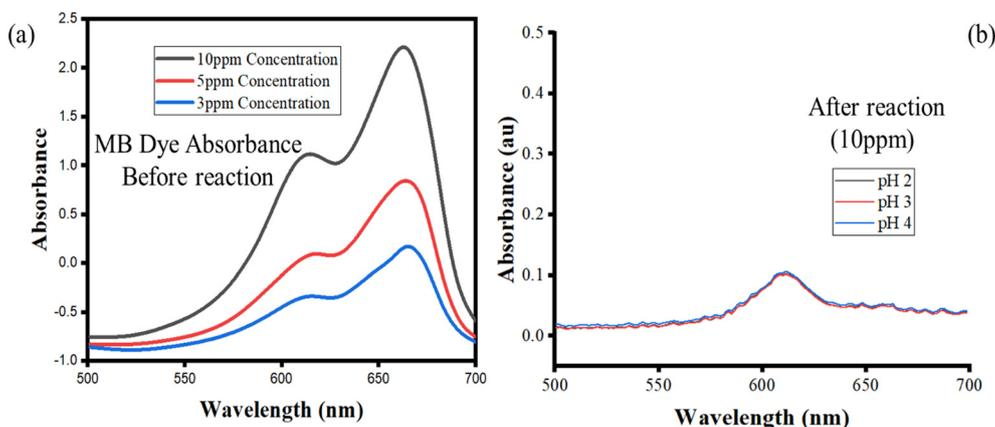
Fig. 16 MB dye adsorption spectra before (a) and after (b) exposure to SiO<sub>2</sub>–TiO<sub>2</sub>–nZVI nanocomposites.
