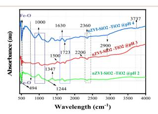
Fig. 6 FTIR analysis of  $nZVI-SiO_2-TiO_2$  nanocomposites synthesized at different pH values (2, 3 and 4).
