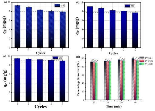
Fig. 12 Sorption capacities of MB dye by  $SiO_2 - TiO_2 - nZVI$  nanocomposites after five successive cycles: (a)  $SiO_2 - TiO_2 - nZVI$  at pH 4, (b)  $SiO_2 - TiO_2 - nZVI$ at pH 3, (c) SiO2-TiO2-nZVI at pH 2 and (d) percentage MB removal per time in the first three regenerative cycles.
