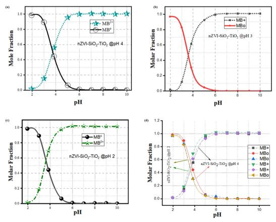
Fig. 17 Speciation behaviour of methylene blue dye following SiO<sub>2</sub>-TiO<sub>2</sub>-nZVI interaction under varying pH conditions: (a) pH 2, (b) pH 3, (c) pH 4, and (d) combined variable pH conditions, with an initial concentration of  $C_0 = 10$  g L<sup>-1</sup>.
