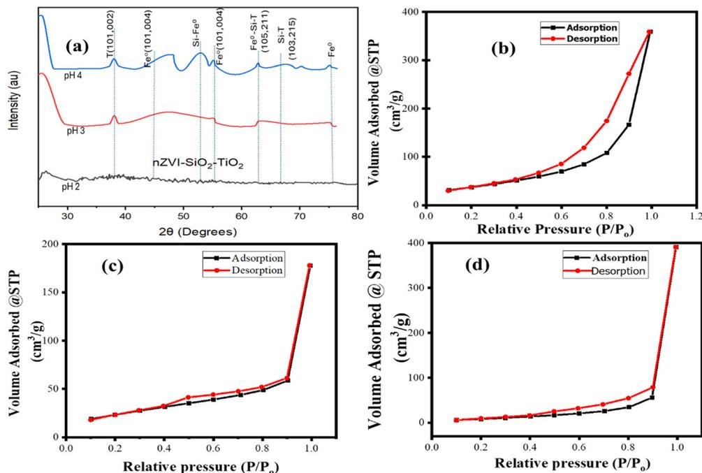
Fig. 4 XRD and BET analysis of nZVI-SiO<sub>2</sub>-TiO<sub>2</sub>. (a) XRD stacked plots of nZVI-SiO<sub>2</sub>-TiO<sub>2</sub> at different pH levels. (b) Adsorption-desorption isotherms at pH 2. (c) and (d) Adsorption-desorption isotherms at pH 3 and pH 4, respectively.
