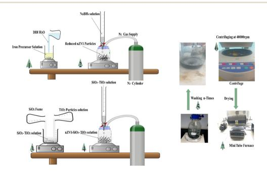
Fig. 1 Graphical representation of the nZVI-SiO<sub>2</sub>-TiO<sub>2</sub> adsorbent fabrication setup.
