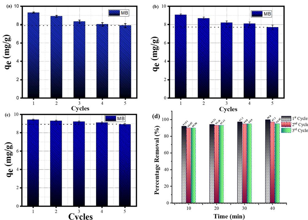
Fig. 12 Sorption capacities of MB dye by SiO<sub>2</sub>-TiO<sub>2</sub>-nZVI nanocomposites after five successive cycles: (a) SiO<sub>2</sub>-TiO<sub>2</sub>-nZVI at pH 4, (b) SiO<sub>2</sub>-TiO<sub>2</sub>-nZVI at pH 3, (c) SiO<sub>2</sub>-TiO<sub>2</sub>-nZVI at pH 2 and (d) percentage MB removal per time in the first three regenerative cycles.
