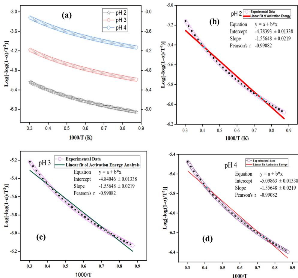
Fig. 11 TGA activation energy analysis of nZVI–SiO<sub>2</sub>–TiO<sub>2</sub> (a), linear fit at pH 2, (b) linear fit at pH 3 and (c) linear fit at pH 4 (d).
