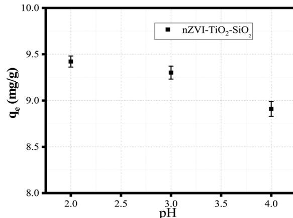
Fig. 13 Influence of synthesis pH on the equilibrium adsorption,  $q_e$  (mg g<sup>-1</sup>), of SiO<sub>2</sub>-TiO<sub>2</sub>-nZVI nanocomposites.
