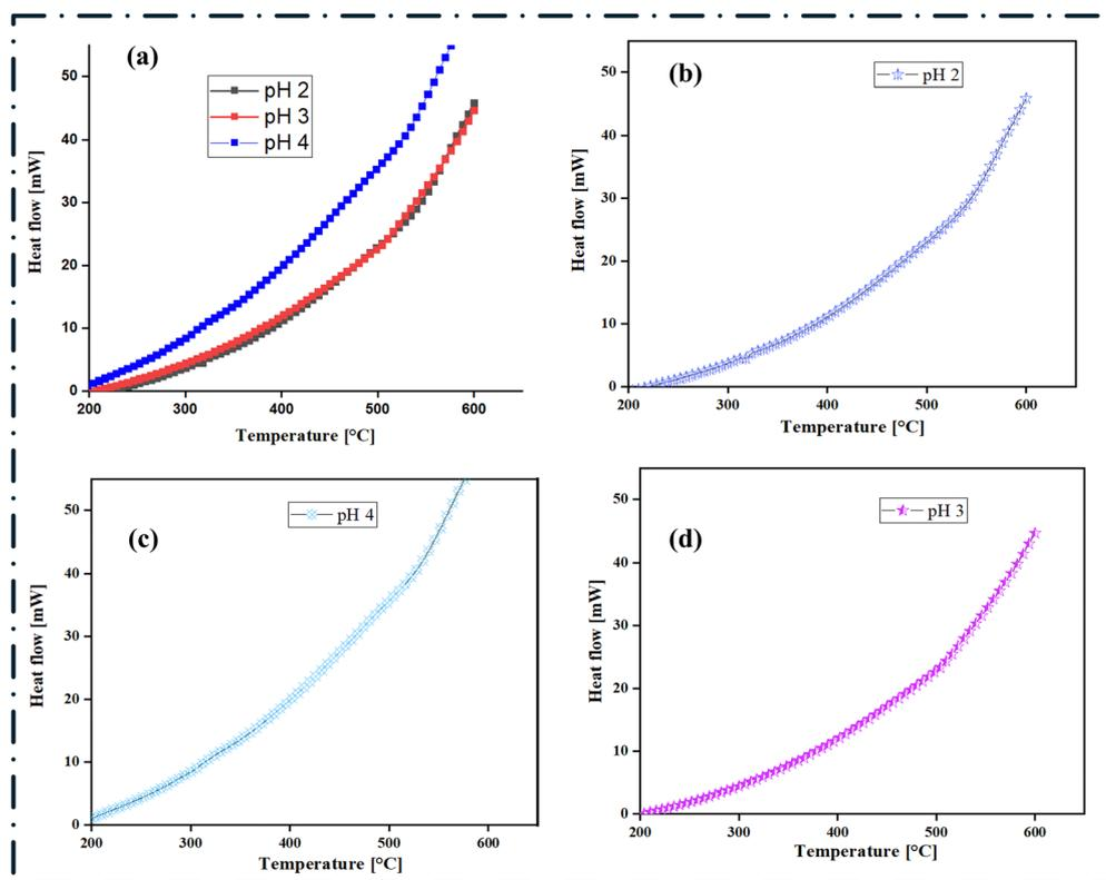
Fig. 7 Differential scanning calorimetry (DSC) analysis of SiO<sub>2</sub>–TiO<sub>2</sub>–nZVI nanocomposites synthesized under different pH conditions. (a) Stacked comparison of the thermal behaviour of SiO<sub>2</sub>–TiO<sub>2</sub>–nZVI under all three reaction conditions; (b) thermal behaviour of SiO<sub>2</sub>–TiO<sub>2</sub>–nZVI at pH 2; (c) thermal behaviour of SiO<sub>2</sub>–TiO<sub>2</sub>–nZVI at pH 3 and (d) thermal behaviour of SiO<sub>2</sub>–TiO<sub>2</sub>–nZVI at pH 4.
