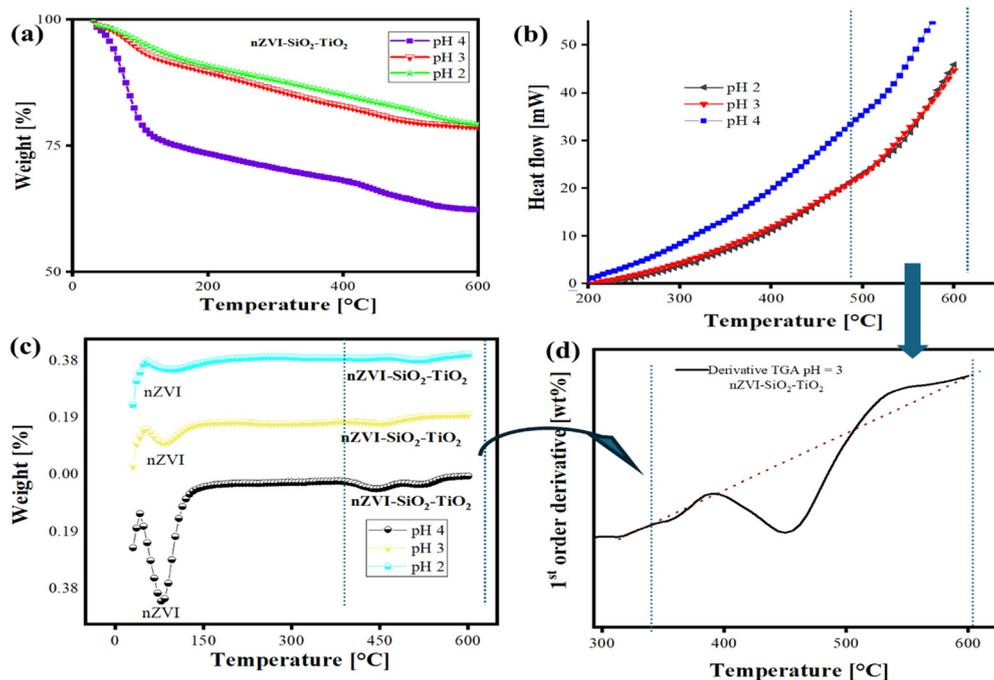
Fig. 8 Thermogravimetric analysis (TGA) and comparison of the thermal properties and characteristics of nZVI-SiO<sub>2</sub>-TiO<sub>2</sub> nanocomposites. (a) Stacked TGA plots, (b) stacked DSC plots and (c) and (d) TGA weight percent derivatives.
