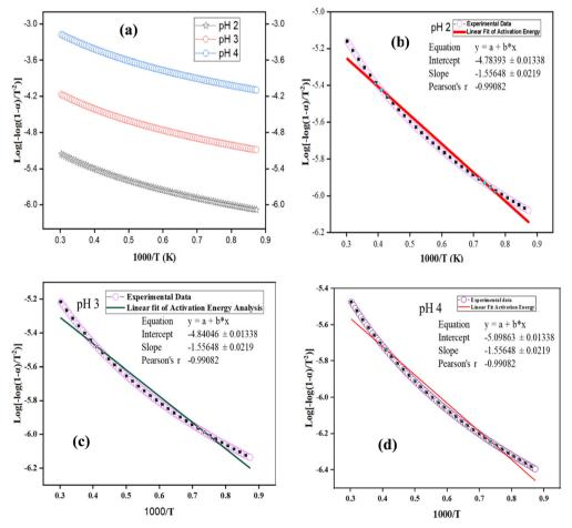
Fig. 11 TGA activation energy analysis of nZVI-SiO<sub>2</sub>-TiO<sub>2</sub> (a), linear fit at pH 2, (b) linear fit at pH 3 and (c) linear fit at pH 4 (d).
