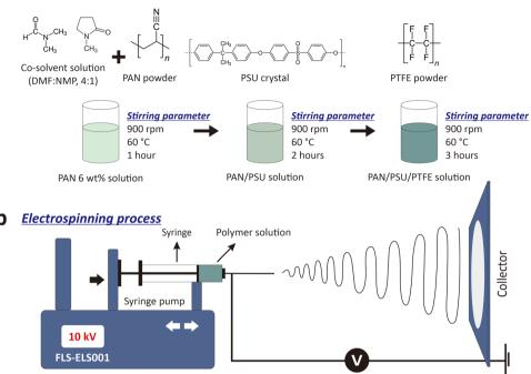
Fig. 1 Solution synthesis and electrospinning processes to fabricate composite nanofibers. (a) Three different solutions were prepared, i.e., polyacrylonitrile (PAN), polyacrylonitrile/polysulfone (PAN/PSU), and polyacrylonitrile/polysulfone/polytetrafluoroethylene (PAN/PSU/PTFE). (b) These solutions were transformed into nanofibers using an electrospinning machine. The parameters used in the electrospinner were a voltage of 10 kV and a tip-to-collector distance of 15 cm.
