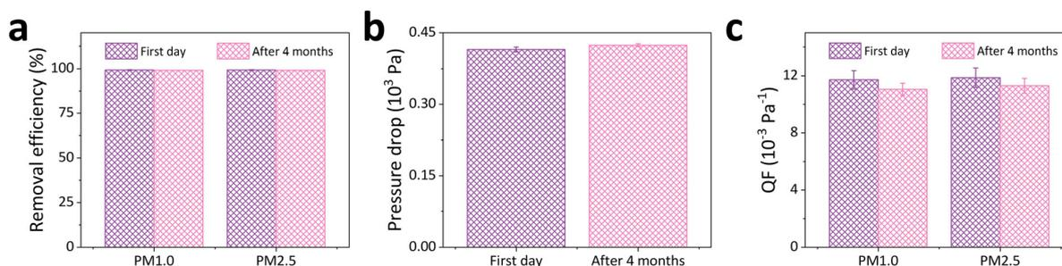
Fig. 6 Durability of the fabricated PAN/PSU/PTFE.2 as a PM filtration membrane. The investigated parameters to assess the membrane durability include (a) removal efficiency, (b) pressure drop, and (c) QF after 4 months. After 4 months, the membrane experienced an insignificant decrease in removal efficiency and an increase in pressure drop. Thus, there was a decrease in QF for both PM<sub>1.0</sub> and PM<sub>2.5</sub>.
