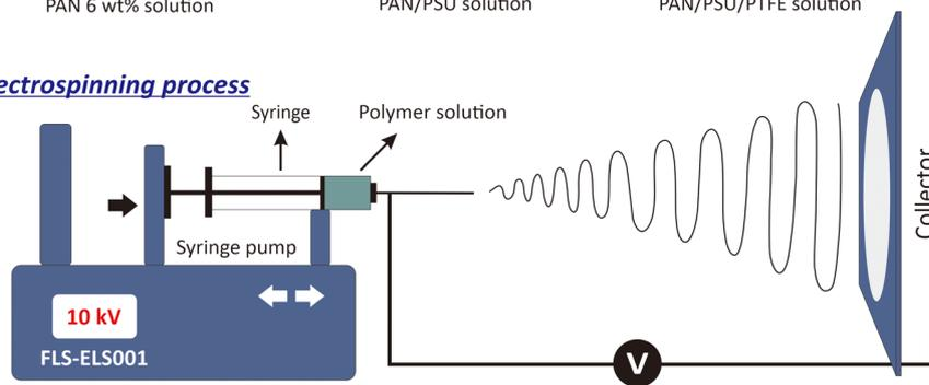
**Fig. 1** Solution synthesis and electrospinning processes to fabricate composite nanofibers. (a) Three different solutions were prepared, *i.e.*, polyacrylonitrile (PAN), polyacrylonitrile/polysulfone (PAN/PSU), and polyacrylonitrile/polysulfone/polytetrafluoroethylene (PAN/PSU/PTFE). (b) These solutions were transformed into nanofibers using an electrospinning machine. The parameters used in the electrospinner were a voltage of 10 kV and a tip-to-collector distance of 15 cm.
