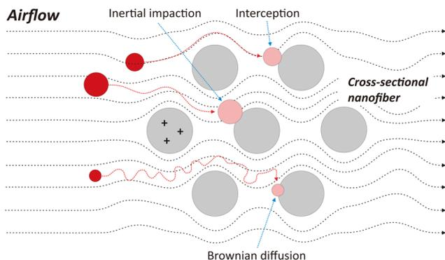
**Fig. 7 PM filtration mechanism.** Common filtration mechanisms that occur between a nanofiber and PM include interception (PM size of 0.1–1  $\mu\text{m}$ ), inertial impaction (PM size of 1–10  $\mu\text{m}$ ), and Brownian diffusion (PM size of < 0.1  $\mu\text{m}$ ).
