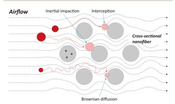
Fig. 7 PM filtration mechanism. Common filtration mechanisms that occur between a nanofiber and PM include interception (PM size of  $0.1-1 \mu m$ ), inertial impaction (PM size of  $1-10 \mu m$ ), and Brownian diffusion (PM size of  $< 0.1 \mu m$ )
